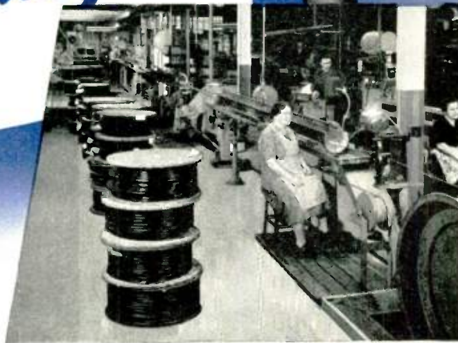
Clean, smooth, properly centered polyethylene covered wire is extruded by this machine.
