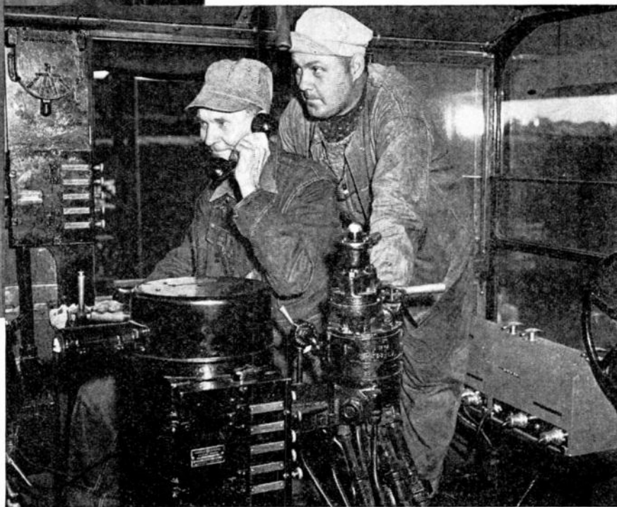
FIRST OF THE ROCK ISLAND'S 2-WAY FM INSTALLATIONS ARE FOR USE BETWEEN DISPATCHER'S OFFICE AND SWITCHING ENGINES. CONVENTIONAL METHOD IS TO SEND COURIERS ON FOOT TO DELIVER MESSAGES TO THE ENGINEERS
