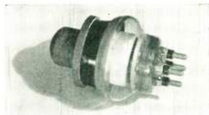
The Machlett 880 is a radio oscillator tube for use in transmitters, and has a maximum output of 60 KW.
