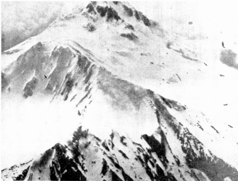
FIG. 1. REPRODUCED FROM FACSIMILE RECEPTION ON FILM AT 96 LINES PER INCH. NOTE THE EXCELLENT CONTRAST
