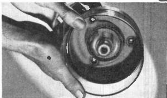
There are four complicated glass to metal seals in this vacuum tube part
