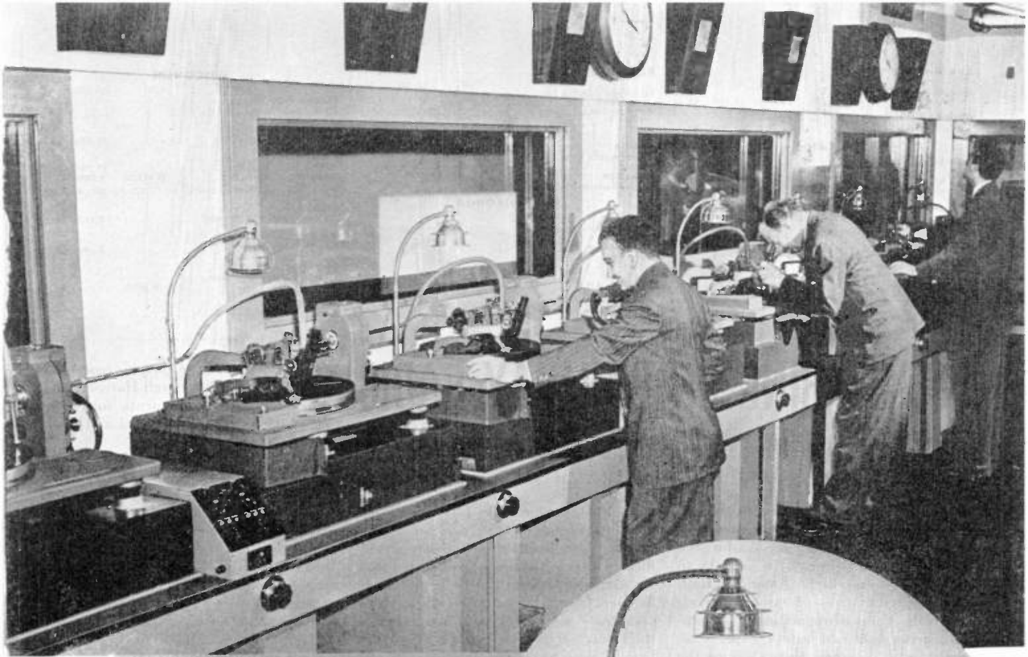
Pictured here is the recording lathe bank at OWI Headquarters, New York City. These RCA recorders are used in making transcriptions of OWI news and entertainment programs for overseas broadcasting.
