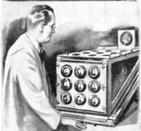
Simpson Vibration Test —Specially designed equipment provides rapid movement of instruments in three different planes. Variable speed regulator permits vibration of any desired intensity.
