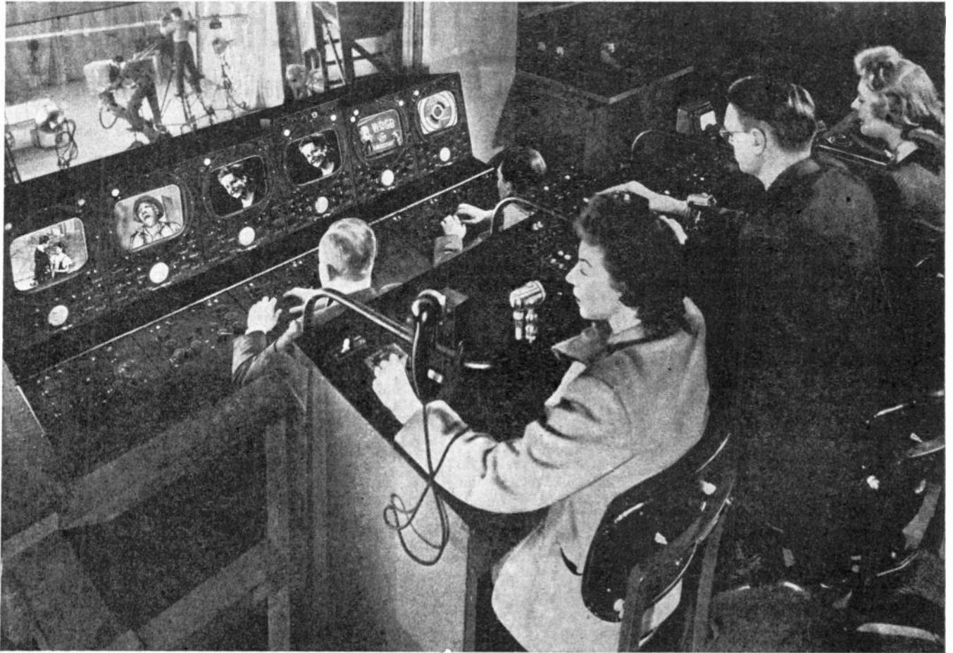
FIG. 9. THE PRODUCER, VIDEO OPERATOR, AND AUDIO OPERATOR, AT THE RIGHT, LOOK INTO THE STUDIO OVER THE HEADS OF THE OPERATORS WHO HANDLE THE CONTROLS OF THE CAMERA AND LINE MONITORS, AND THE SHADING DESK
