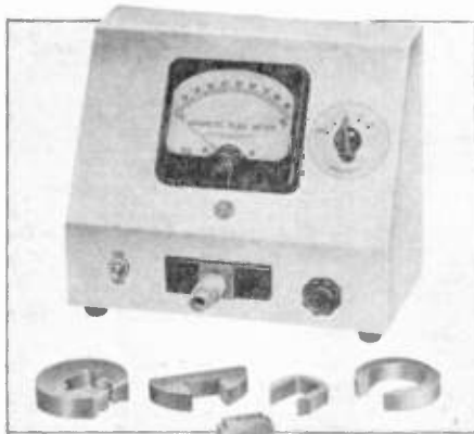
FIG. 6. FLUX METER FOR TESTING MAGNETS
