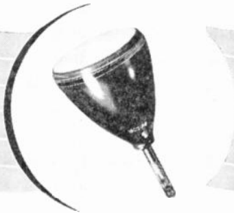
2. THE KINESCOPE — The reproducing tube used in all present-day receivers. Developed by Dr. V. K. Zworykin of RCA Laboratories as part of his "all-electronic" television system.
