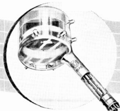
1. THE ICONOSCOPE —The "electric eye" of the television camera. Developed by Dr. V. K. Zworykin, RCA scientist, and brought to a high degree of perfection by RCA engineers.
