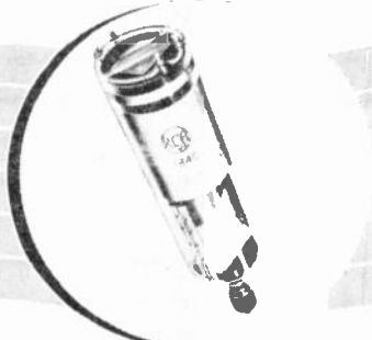
3. THE "ORTHICON" — The high-sensitivity pickup tube, which requires much less light and hence makes outside pickups practical. Developed by Dr. Rose and Dr. Iams of RCA Laboratories.
