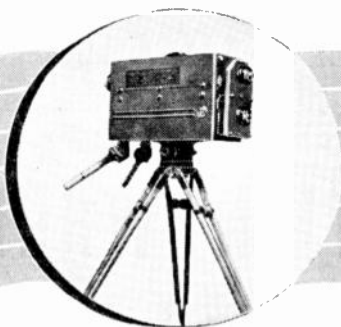
5. THE FIELD CAMERA — The RCA field pickup camera shown here is the first camera to use the "orthicon" pickup tube—by far the most satisfactory for "outside" pickups.
