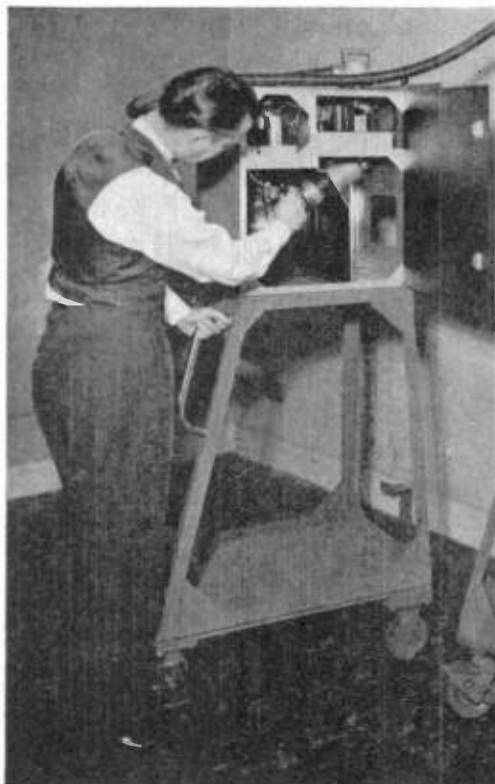
FIG. 16. FILM PICKUP CAMERA IN POSITION. FIG. 15. STANDARD FILM PROJECTORS MODIFIED FOR TELEVISION TRANSMISSION OF MOTION PICTURES
