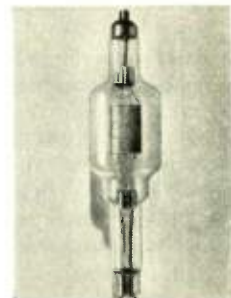
ML-100, high-voltage industrial rectifier.
