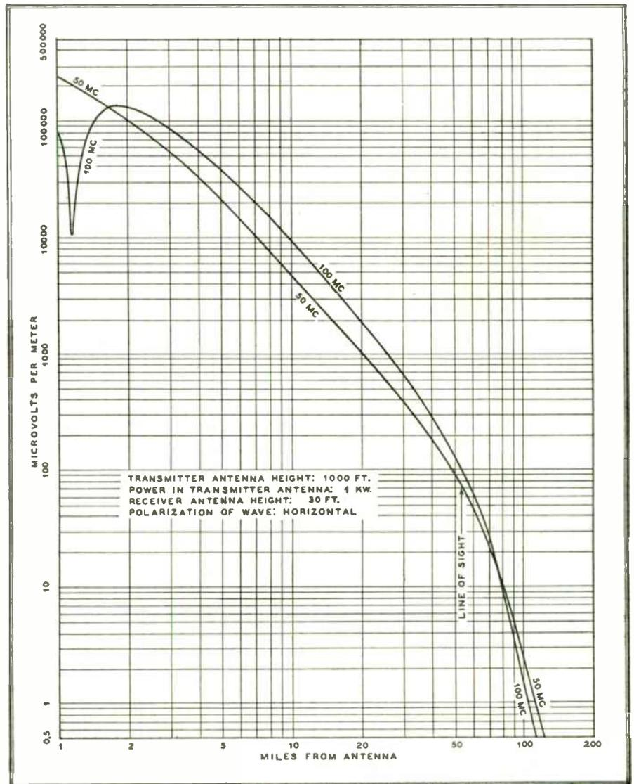
FIG. 8. FIELD STRENGTH AS A FUNCTION OF DISTANCE AT VERY HIGH FREQUENCIES
