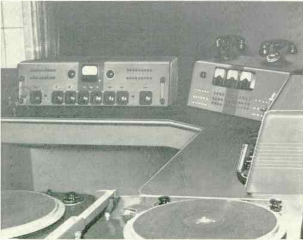
*Left*—The control room in the studios shared by FM station WSBF and AM station WSBT. Two RCA 76-B2 Consolettes handle the output of two studios. A master control console (center) provides monitoring and switching of outgoing lines to the two transmitters. The RCA 70-C Turntables may be seen in the foreground. In the studios RCA 44-BX Microphones are used.
