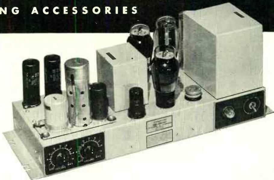
**THE 108 SERIES** consist of four different amplifiers available simply by changing one or two small input panels on the master chassis. Except for these input panels all amplifiers have the same transmission characteristics. Input impedance, gain and noise level depending on types listed below.
