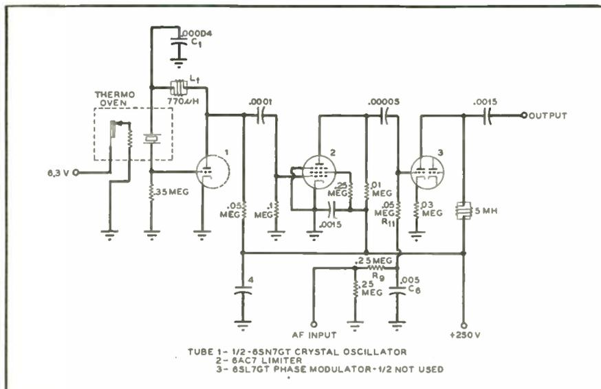
FIG. 7. CRYSTAL OSCILLATOR AND PHASE SHIFT CIRCUITS OF THE TRANSMITTER
