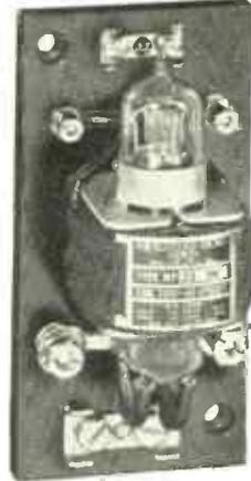
However, mercury-plunger relays by H-B Electric are not limited to tube applications but may be used for practically any timing, load or control circuit. They are available for a-c up to 440 volts and for d-c up to 250 volts, with contact capacities as high as 30 amperes. All have hermetically sealed mercury-to-mercury contacts which are positive,
