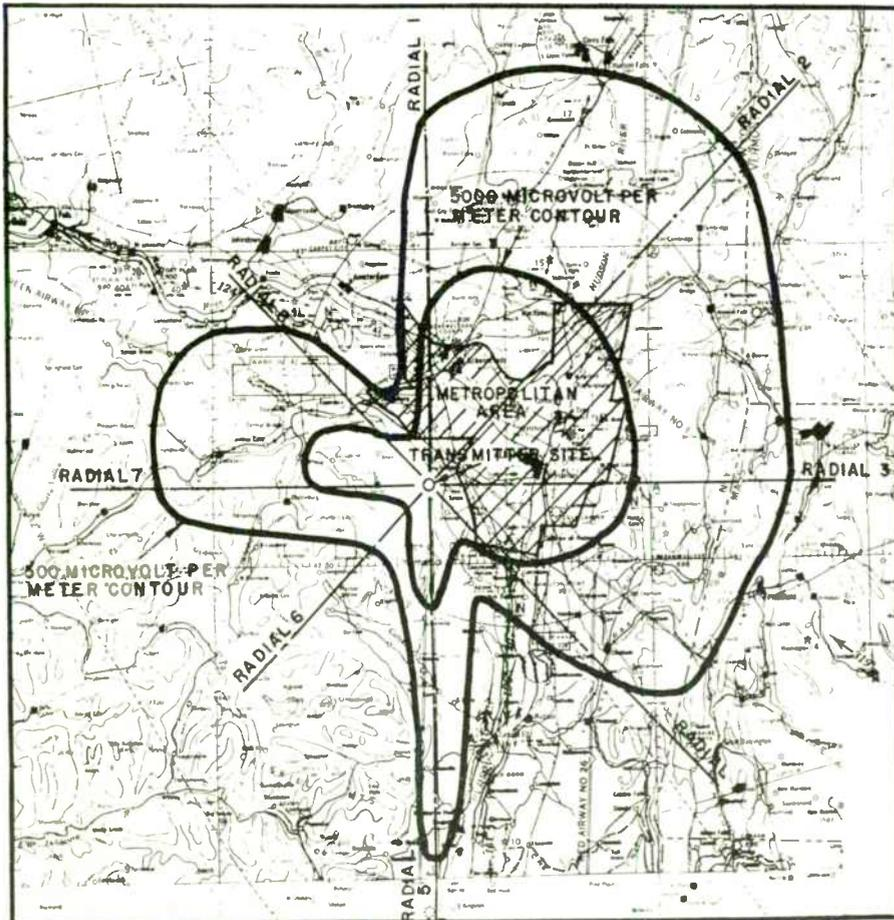
FIG. 33. CALCULATED 500- AND 5,000-MICROVOLT CONTOURS OF TELEVISION STATION WRGB
