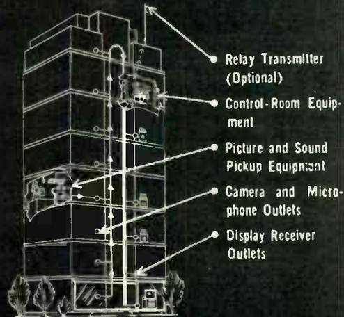
A typical G-E Intra-Tel system. With the Intra-Tel system, portable television cameras and sound microphones can be operated from any place in store or plant. Pictures and sound picked up by cameras (1) and
