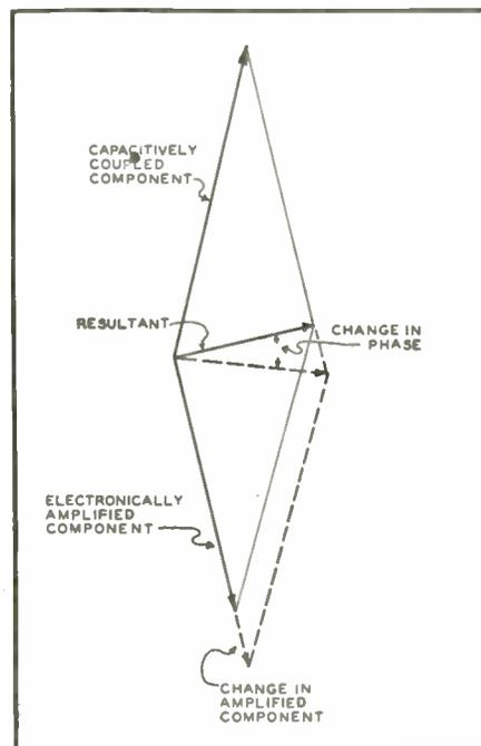
FIG. 8. HOW MODULATION IS ACCOMPLISHED
