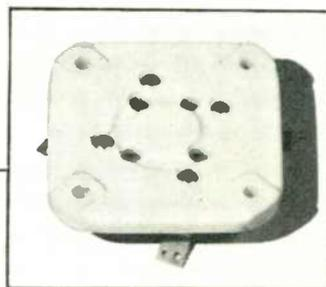
FIG. 8, ABOVE: THE DIMENSIONS OF THIS SOCKET HAVE BEEN REDUCED SUBSTANTIALLY OVER SIMILAR, PRECEDING TYPES
