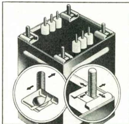
FIG. 10. IMPROVED MOUNTING STUDS
