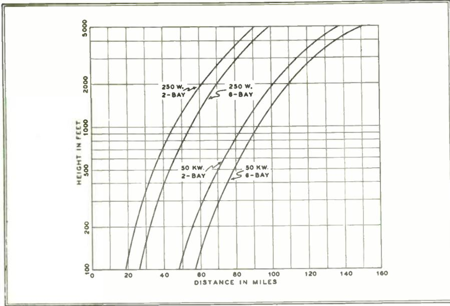
FIG. 9. RELATION OF HEIGHT, POWER, AND DISTANCE TO 50-MICROVOLT CONTOUR
