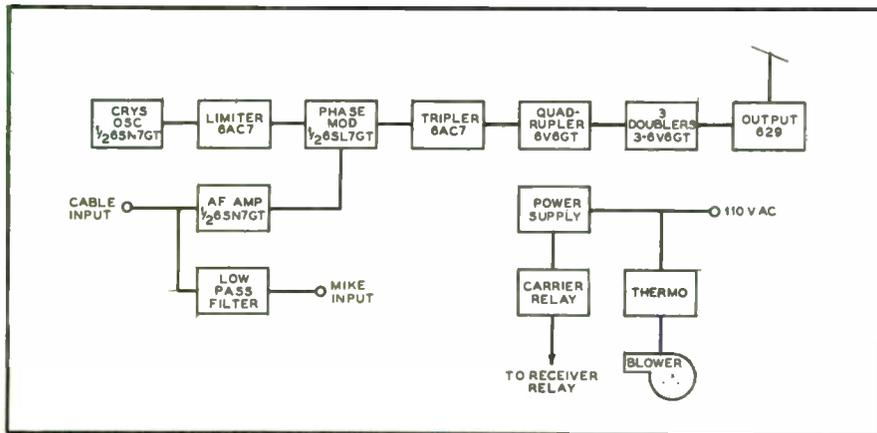
FIG. 6. BLOCK DIAGRAM SHOWING TUBE TYPES AND FUNCTIONS OF THE TRANSMITTER
