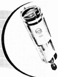
3. THE "ORTHICON" — The high-sensitivity pickup tube, which requires much less light and hence makes outside pickups practical. Developed by Dr. Rose and Dr. Iams of RCA Laboratories.
