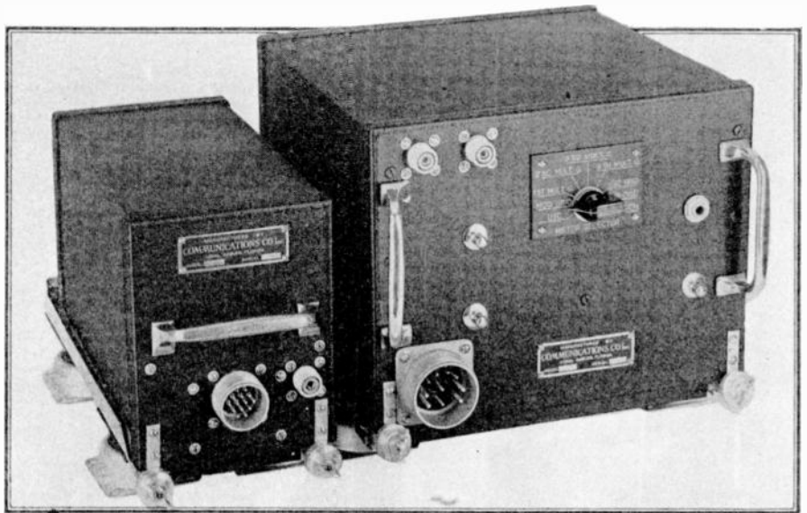
FIG. 1. FM RECEIVER, LEFT, AND TRANSMITTER FOR 15, 25, OR 50W. OUTPUT
