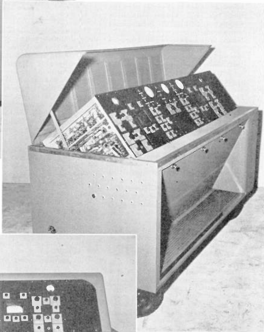
FIG. 3, RIGHT. LOUVERS IN THE COVER, BEHIND THE CONTROL PANEL, PROVIDE AN OUTLET FOR AIR FORCED UPWARD BY FANS AT THE BOTTOM
