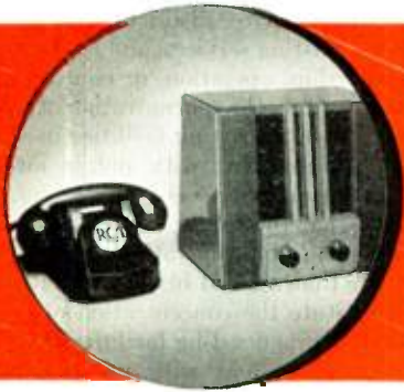
9. Station Handset and Control Unit: Furnished with the FM Station Transmitters shown here. The control unit contains a loudspeaker, plus controls for adjustment of "volume" and "squench." Also, "transmit," "receive," and "stand-by" signal lights.
