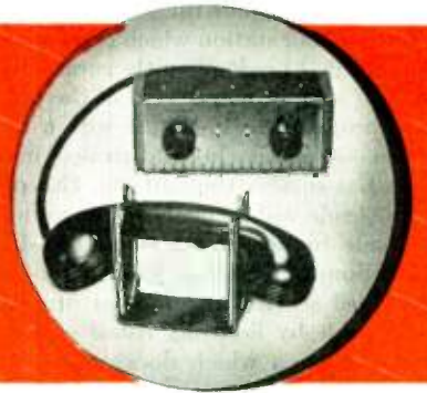
10. Mobile Handset and Control Unit: Furnished with the FM Mobile transmitters shown above. The two units can be conveniently mounted on the dash in any desired position. Control includes "volume" and "squench." Signal lights indicate "transmit" and "stand-by."
