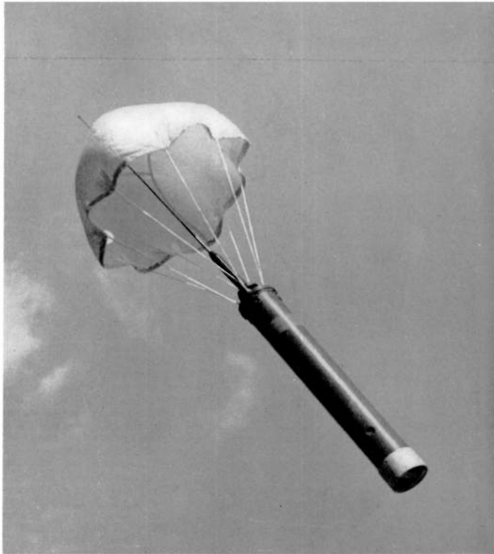
FIG. 1. A SONO-BUOY FM TRANSMITTER FALLING FROM A PLANE TO THE WATER
