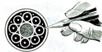
4. Coaxial cable—a single wire strung in a pencil size tube—extended the usable frequency band up to millions of cycles per second and today carries hundreds of messages per circuit, or the wide bands needed for television.
