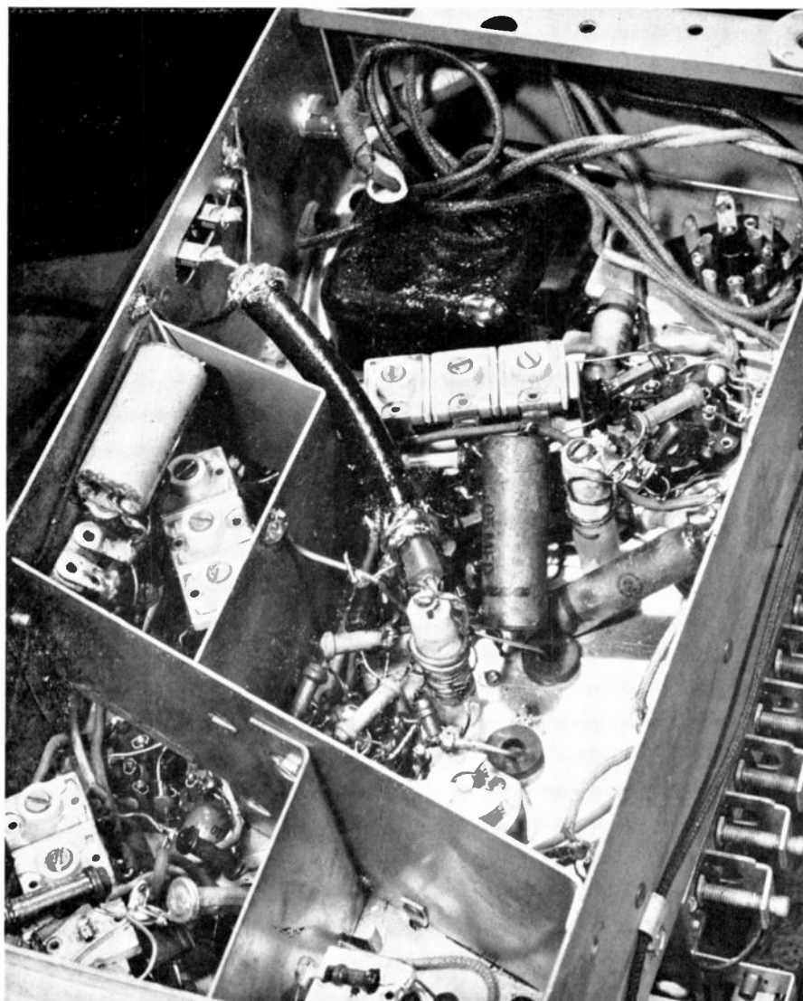
FIG. 1. CHASSIS OF THE TRANSLATOR AFTER CHANGES FOR HIGH BAND OPERATION
