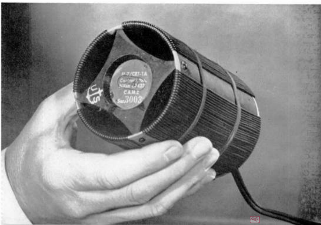
FIG. 2. THIS MAGNETO-STRICTION MICROPHONE LISTENED TO SUBMARINES
