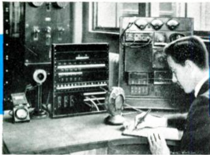
1922. One of the earliest audio systems, shown here at WWJ, Detroit, used a Western Electric 8-type amplifier, with keys, jacks and plugs provided for line selection and output switching.
