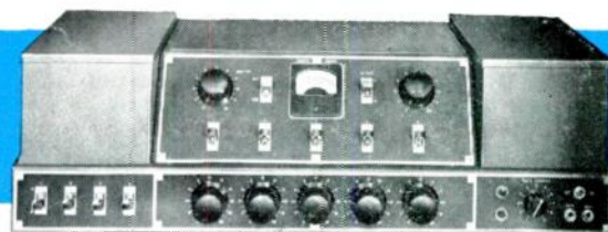
1936. The all a-c, console type, self-contained 23A studio control equipment introduced a brand new style for standardized studio units. First studio system to use stabilized feedback. The current 23C, with frequency response to 15,000 cycles, is widely used in AM and FM broadcasting.
