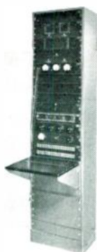
1931. This smartly styled 9A audio equipment was the first all a-c system. All controls in a single panel; frequency response stepped up to 10,000 cycles.
