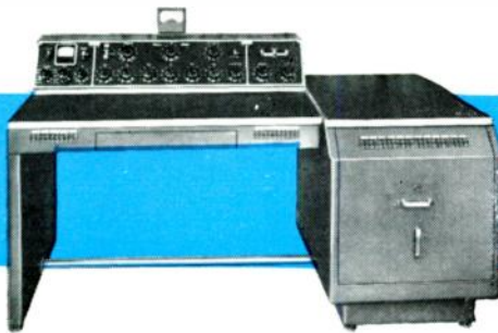
1939. This custom-built audio console for WOR was the first commercial type meeting all requirements for FM use. It provided circuits and equipment to meet specific operating conditions. The tailored metal desks mounted amplifiers, control and switching equipment and turntable units—all within easy reach of the operator.
