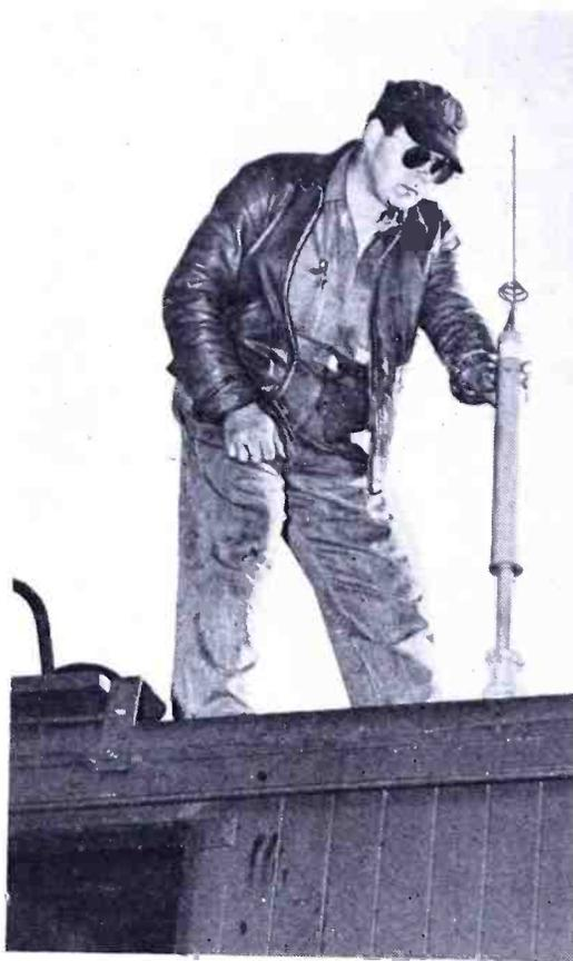
FIG. 4. ANTENNA USED IN CONJUNCTION WITH THE CABOOSE TRANSMITTER-RECEIVER
