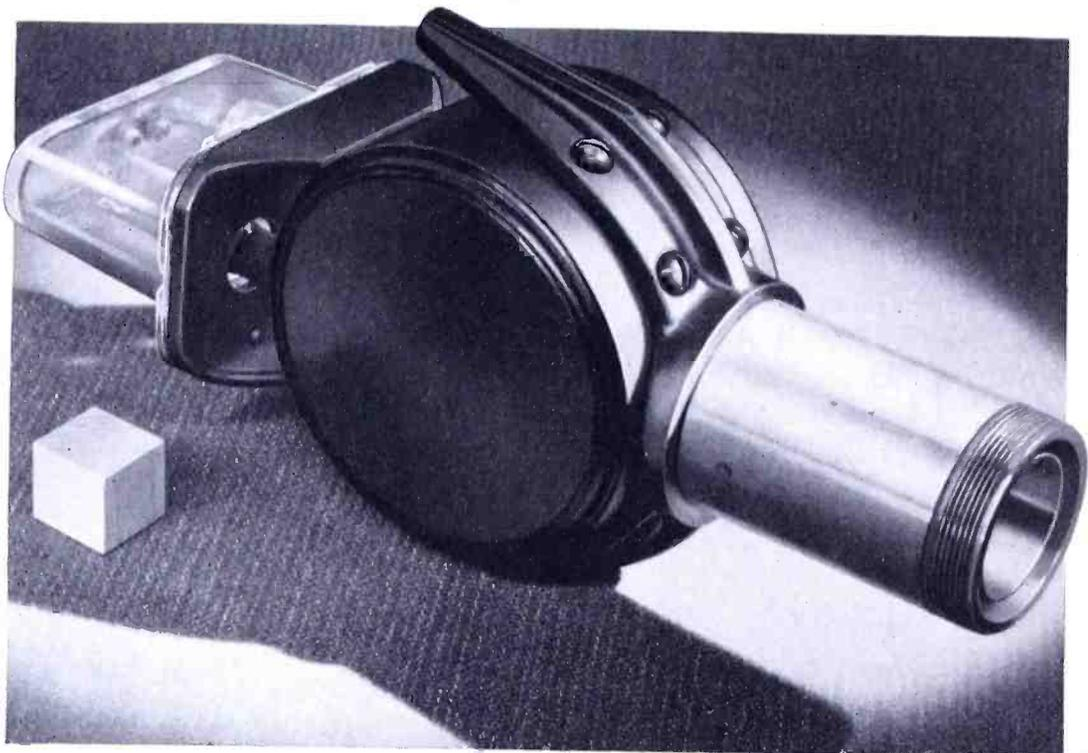
FIG. 48. An external view of a 728A-J magnetron (275 kw., 930 mc.). The concentric cylindrical sleeve to be seen inside the output circuit coupling, from which the magnetron is supported, is a part of the choke, Fig. 47. Note the heavy glass protective housing over the input leads.
