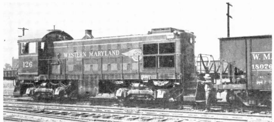
FIG. 4. ONE OF THE DIESEL ENGINES EQUIPPED FOR RADIO, AT PORT COVINGTON, MD.
