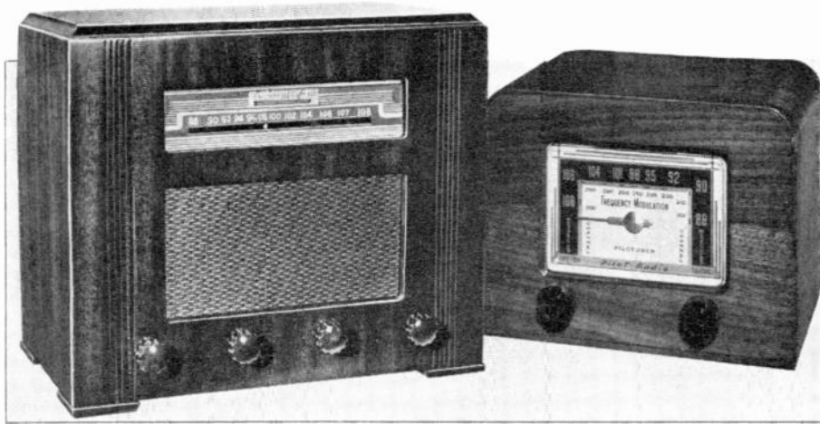
INEXPENSIVE "STARTER" MODELS ARE INTRODUCING MANY LISTENERS TO FM. LEFT: SWITCH ON ELECTRONICS MODEL IS FOR BUILT-IN OR EXTERNAL AMPLIFIER & SPEAKER. RIGHT: PILOT FM TUNER OPERATES THROUGH ANY AM SET
