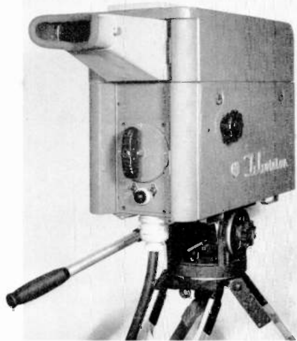
FIG. 5. VIEW OF LENS TURRET AND SIGNAL LIGHTS AT FRONT OF CAMERA. FIG. 6. BIG KNOB AT REAR ROTATES TURRET
