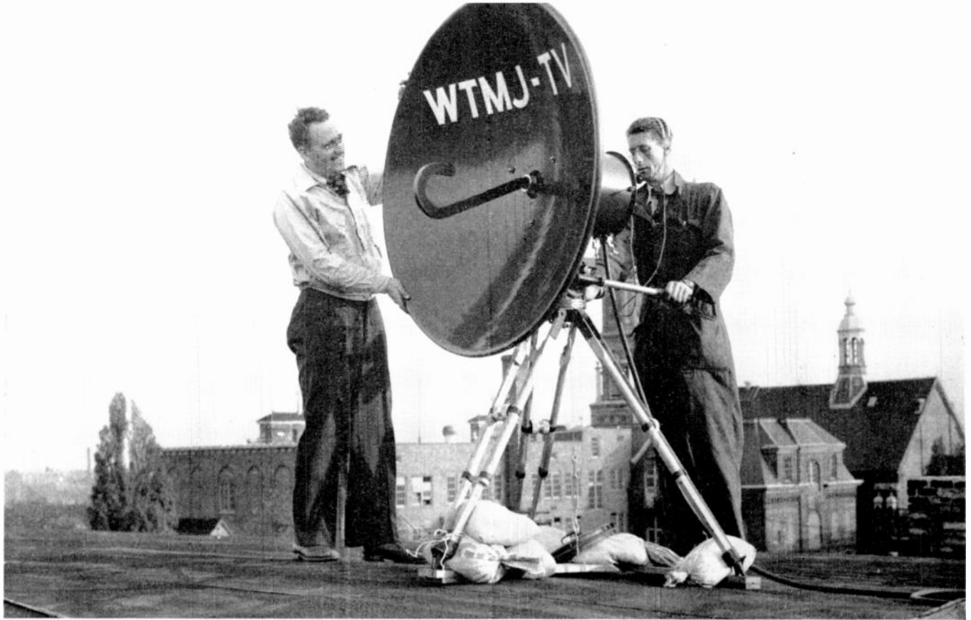
MICROWAVE TELEVISION RELAY ANTENNA, SANDBAGGED TO KEEP IT STEADY IN THE WIND, IS MADE READY FOR REMOTE PICKUP
