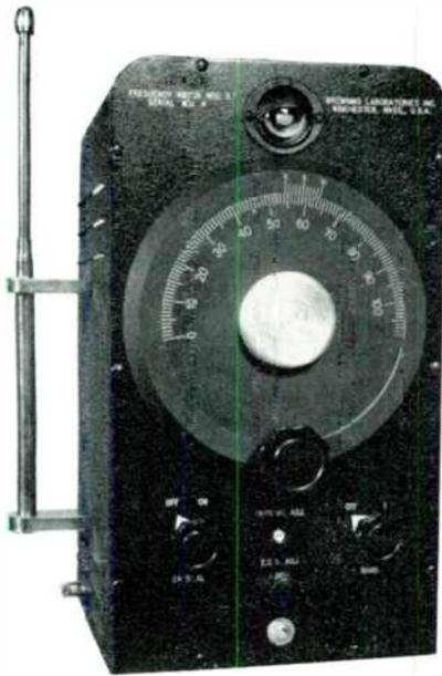
**Model S-4: Calibrated at any 1 to 5 points, 1.5 to 70 mc.**
