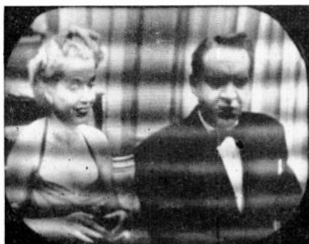
Left, actual photo of WNBW-WNBT co-channel interference. Right, interference pattern eliminated by Kell synchronizing control, developed at RCA Laboratories
