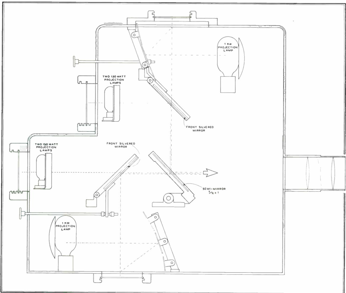
Fig. 1. Two moveable mirrors and the semi-mirror, or optical mixer, permit unlimited combinations of effects from four slides
