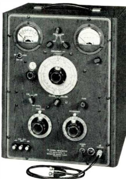
**RF OUTPUT VOLTAGE**—0.2 volt to 0.1 micro-volt. Output impedance 26.5 ohms.
