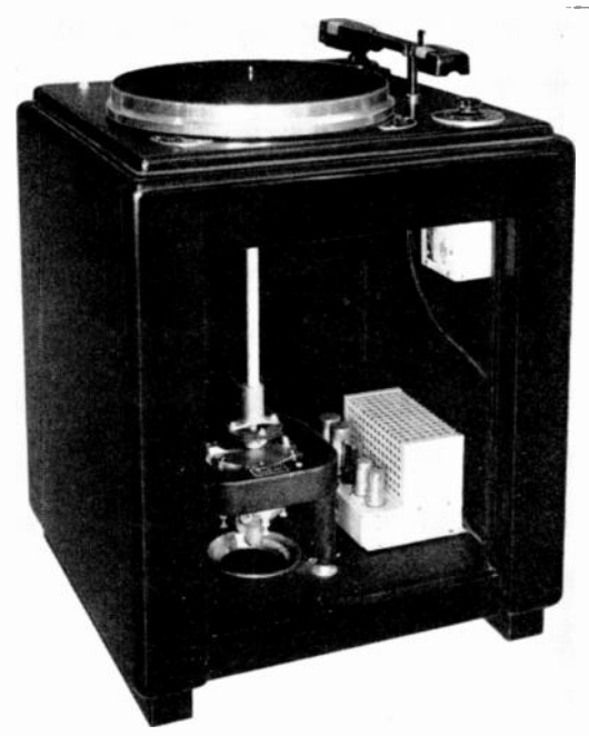
Fig. 6. The Fairchild model 523 recorder provides instantaneous and continuous variation of the cutting pitch. Fig. 7. Transcription turntable has a preamplifier-equalizer at the front right corner of the cabinet
