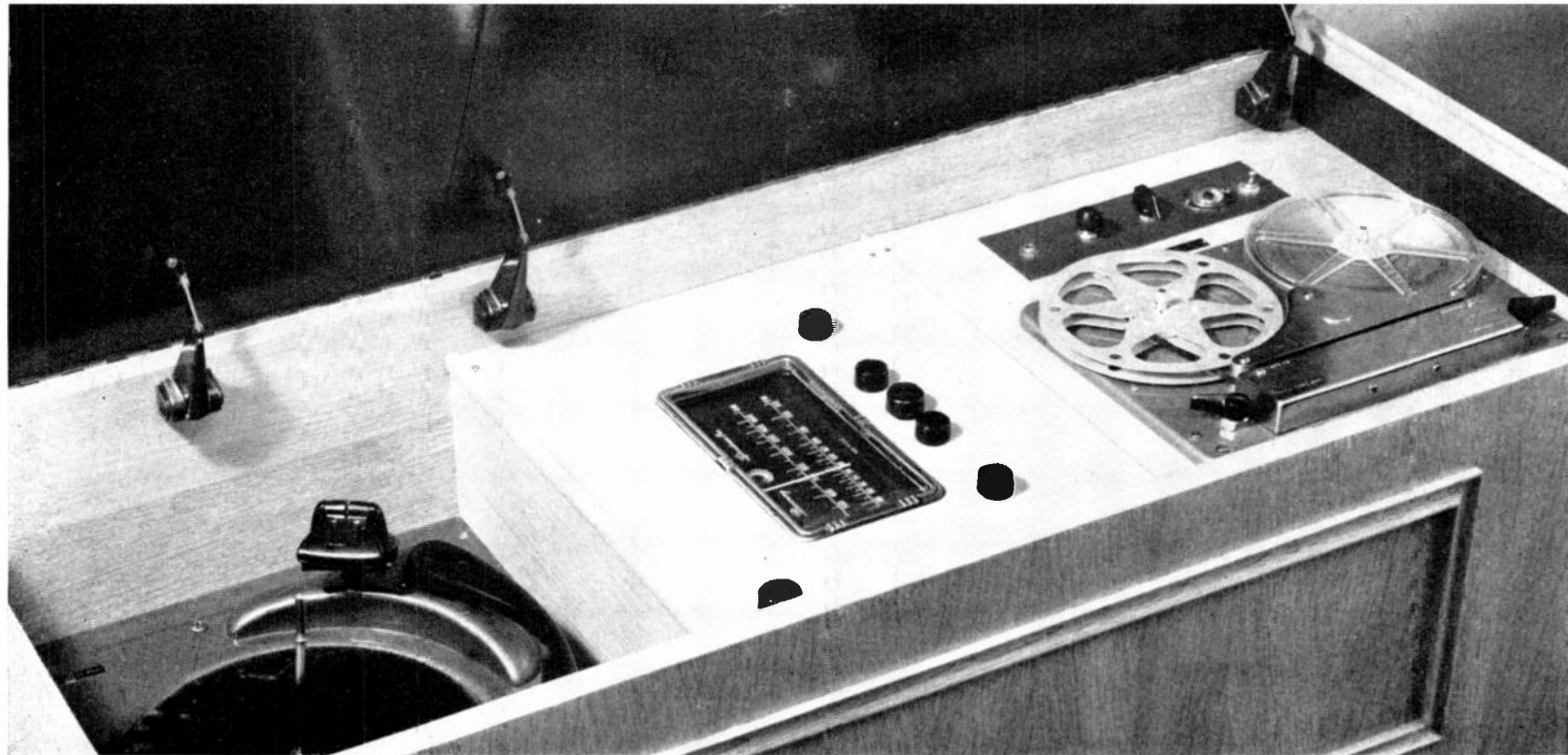
THIS CUSTOM-BUILT INSTALLATION, BY UERIC J. CHILDS, HAS A BROWNING RJ-12A FM-AM TUNER USING THE GENUINE ARMSTRONG FM CIRCUIT
