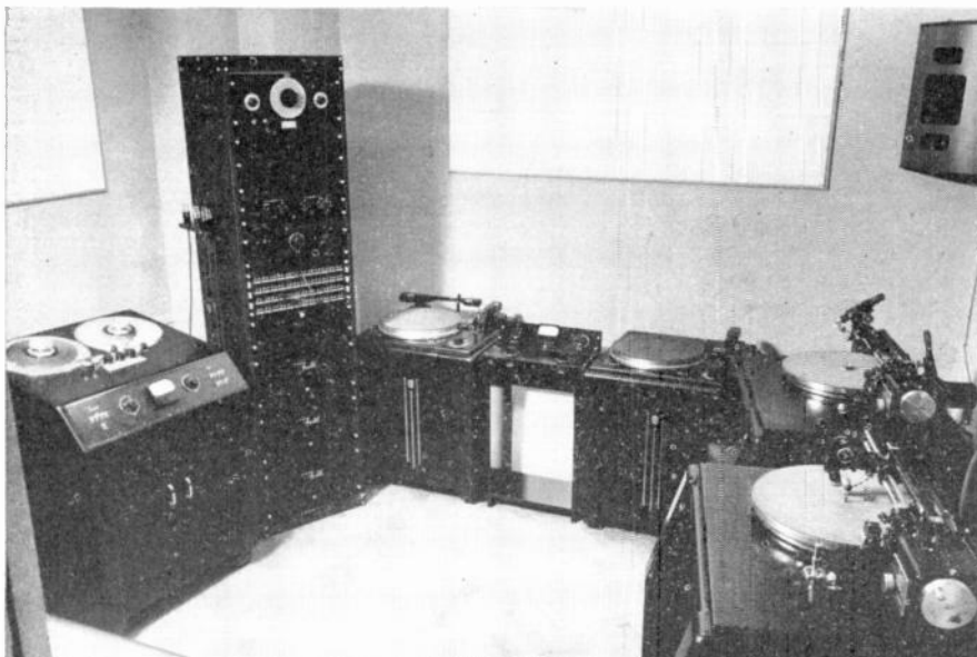
Fig. 2. Cutting-room equipment, in the form of a U, facilitates one-man operation
