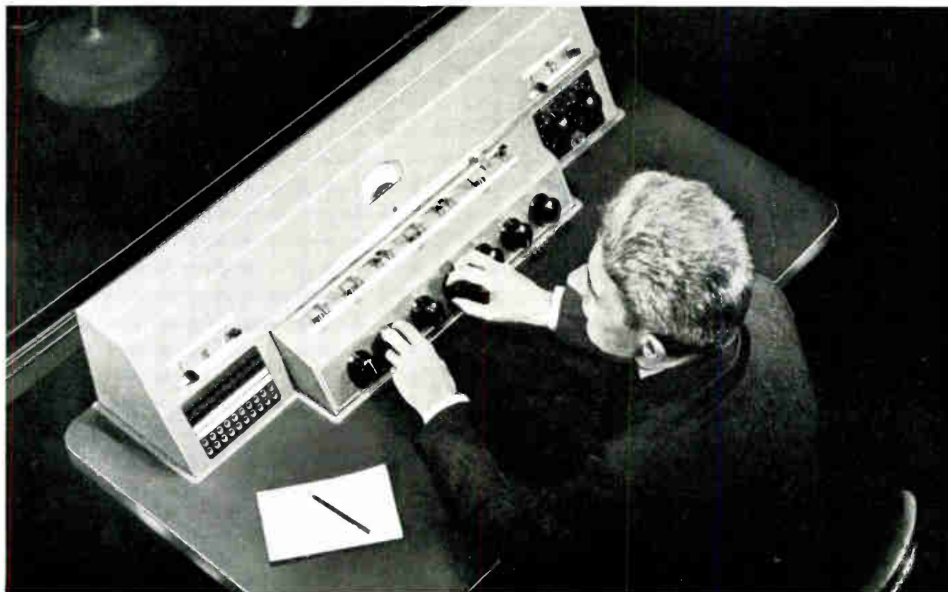
FIG. 2, ABOVE. The seven control knobs across the lower front are, from left to right, line mixer, four microphone mixers, and master gain controls for each of two channels. Talk-back key and line mixer transfer key are above the line mixer.
