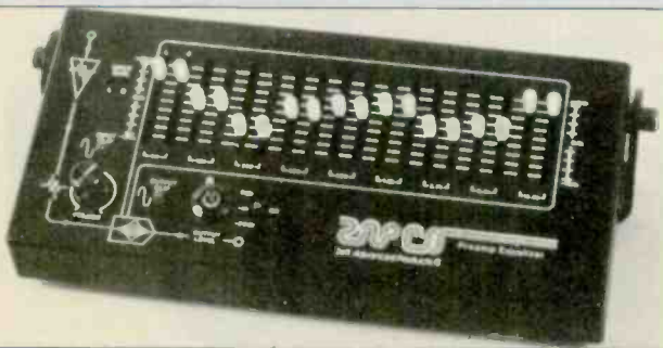
Designed for mounting anywhere, the Zeff PEQ equalizer has 9 bands (50, 100, 200, 400, 800, 1600, 3200, 6400, and 12800 Hz), some unique input and output clipping indicators to help tune-out distortion, and a preamp. $250. Circle 127.
