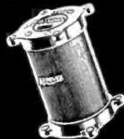
Stack-mounting heavy-duty mica capacitors available in five sizes, 1000 to 35,000 test volts A. C. effective, .00001 to .5 mfd. Intended for such transmitting functions as grid, plate blocking, coupling, tank and by-passing, in those higher-powered installations.
