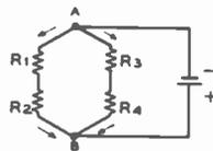
In this type of circuit the resistors are arranged in series groups, and these groups are then placed in parallel.
