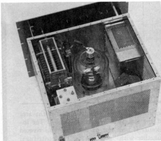
components are removed from the r-f inclosure and are mounted on phenolic terminal boards between the inclosure and the amplifier panel.
