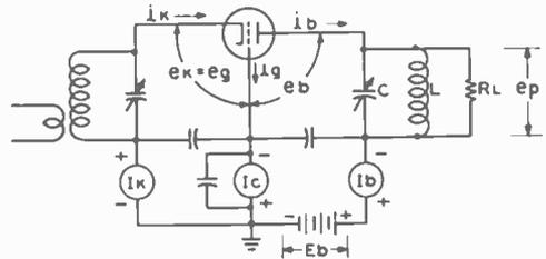
$$\text{PEP POWER TO LOAD} = \frac{(e_b \text{ MIN} + e_g \text{ MAX}) \times i_1 \text{ MAX}}{2}$$
