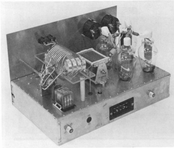
Layout of parts is not critical, provided reasonable care is taken to provide short, direct leads in the plate and filament circuits. The plate tuning capacitor ( $C_6$ ) is centered on the chassis, with the tubes grouped at the corners of a square at one end of the chassis. The plate r-f choke ( $RFC_2$ ) is placed at the center of this square, with the B-plus bypass capacitor mounted immediately beside the choke, atop the chassis.
