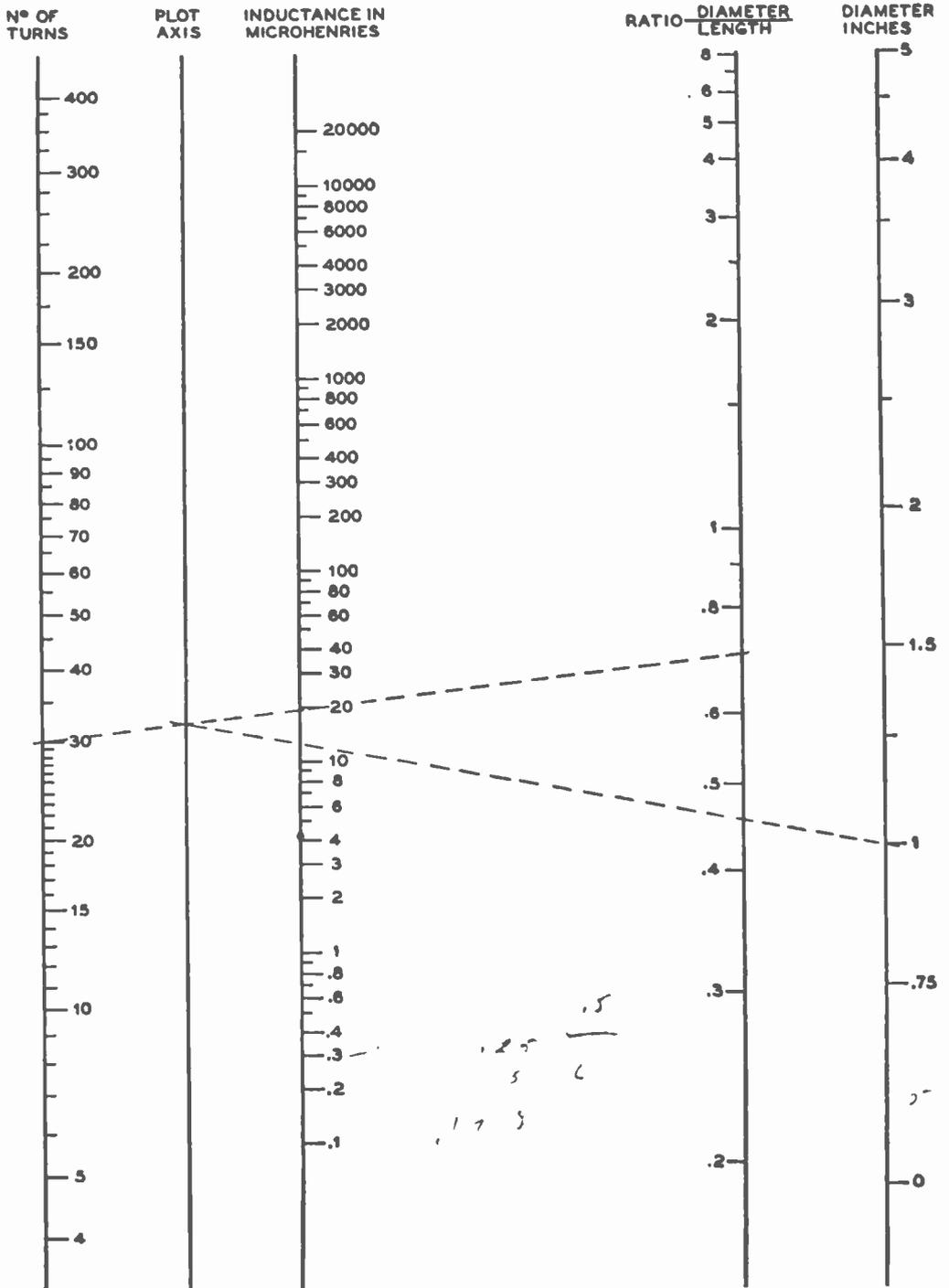
ductance, the D/L ratio, and the diameter are known, simply work backwards from the example given. In all cases, remember that the straightedge reads either turns and D/L ratio, or it reads inductance and diameter. It can read no other combination.
