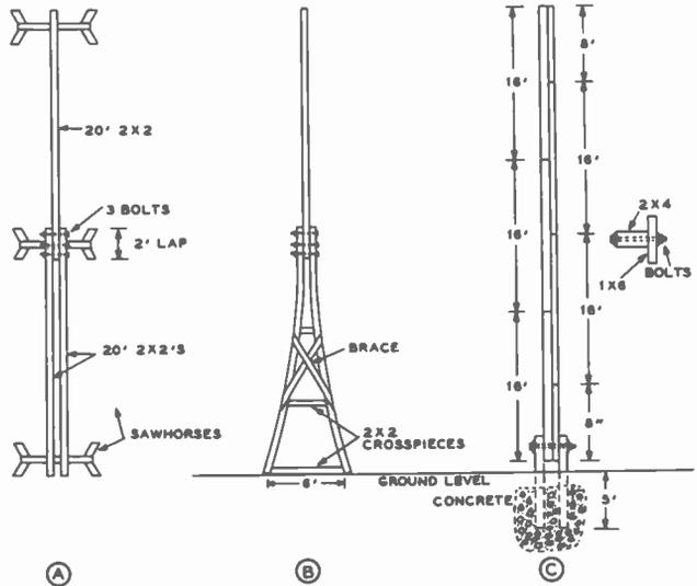
braces and the cross pieces are installed and the assembly given several coats of good-quality paint as a protection against weathering.
