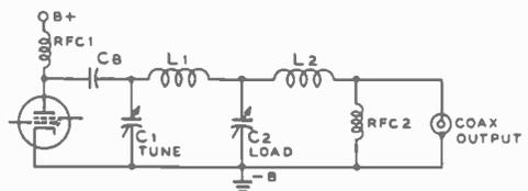
$$PLATE\ LOAD\ (OHMS) = \frac{E_B}{2 \times I_B}$$
