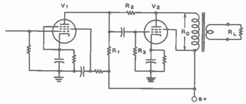
$$\text{DB FEEDBACK} = 20 \text{ LOG} \left\{ \frac{R_2 + R_A (G_{MV2} R_0)}{R_2} \right\}$$
