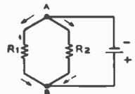
The two resistors  $R_1$  and  $R_2$  are said to be in parallel since the flow of current is offered two parallel paths. An electron leaving point A will pass either through  $R_1$  or  $R_2$ , but not through both, to reach the positive terminal of the battery. If a large number of electrons are considered, the greater number will pass through whichever of the two resistors has the lower resistance.
