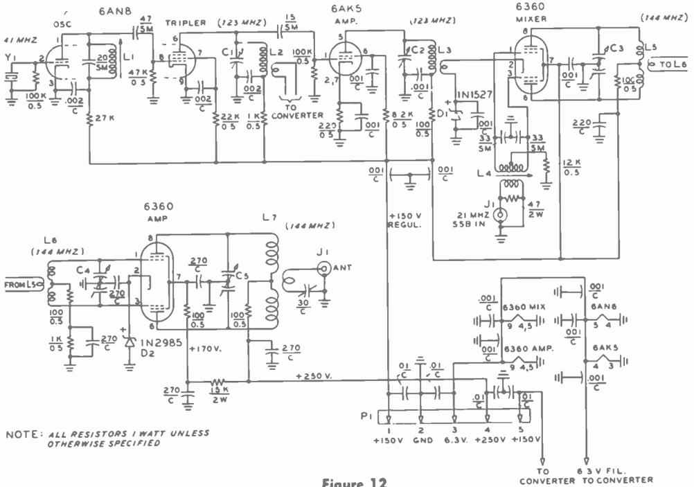
SCHMATIC, TRANSMITTER SECTION OF TRANSVERTER
