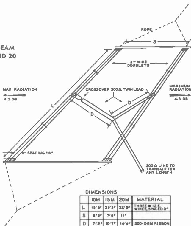
greater directivity gain while maintaining a bidirectional characteristic. However, it must be kept in mind that to realize a worthwhile increase in directivity and gain while maintaining a bidirectional pattern the individual arrays must be spaced sufficiently to reduce the mutual impedances to a negligible value.
