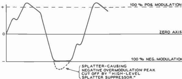
*A high-level splatter suppressor may be used in a transmitter without a clipper-filter to reduce negative-peak clipping, or such a unit may be used following a clipper-filter to allow a higher average modulation level by eliminating the negative-peak clipping which the wave cant caused by phase shift might produce.*
