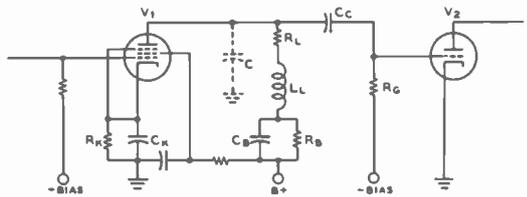
MID-FREQUENCY GAIN =  $G_{M V1} R_L$
