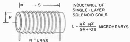
WHERE  $R$  = RADIUS OF COIL TO CENTER WIRE
