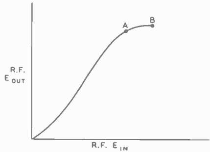
**LINEARITY CURVE OF TYPICAL TETRODE AMPLIFIER**
