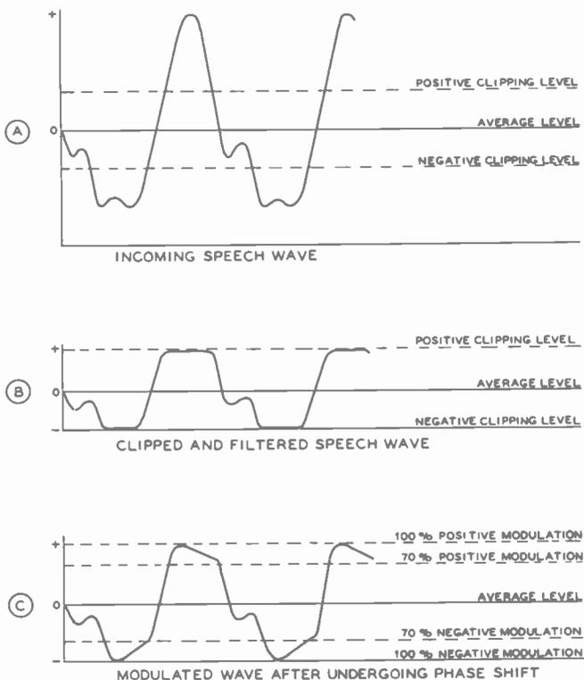
characteristic insofar as it is possible in the stages *following* the clipper-filter. Feeding the plate current to the final amplifier through a choke rather than through the secondary of the modulation transformer will help materially.
