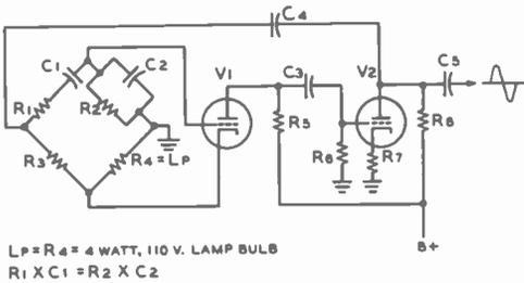
$L_p = R_4 = 4$  WATT, 110 V. LAMP BULB
