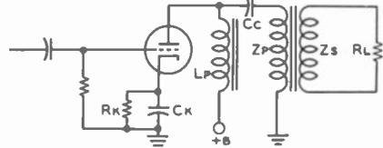
(C) IMPEDANCE-TRANSFORMER COUPLING
