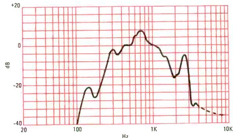
Fig. 3—The frequency-response curve of a typical old-time horn loudspeaker; bad enough, without even considering the distortion! It's of little wonder that dynamic speakers took over so rapidly.
