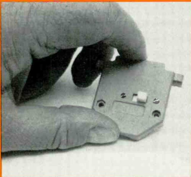
Make certain that the switch's handle is free to move to both extreme positions. If it's not, remove the switch and file the opening to accommodate the switch's handle travel.
