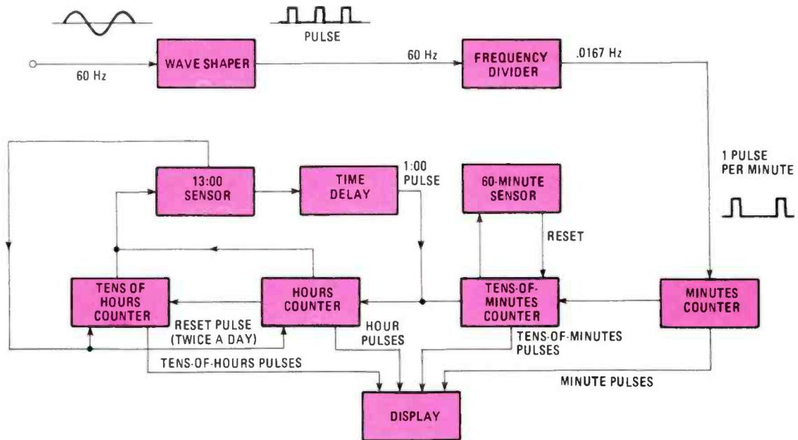
Fig. 1—The block diagram shows the flow of operation of the TTL Clock. Comparing this with the schematic diagram, you can see that the format is the same. That is also true in the foil patterns.
