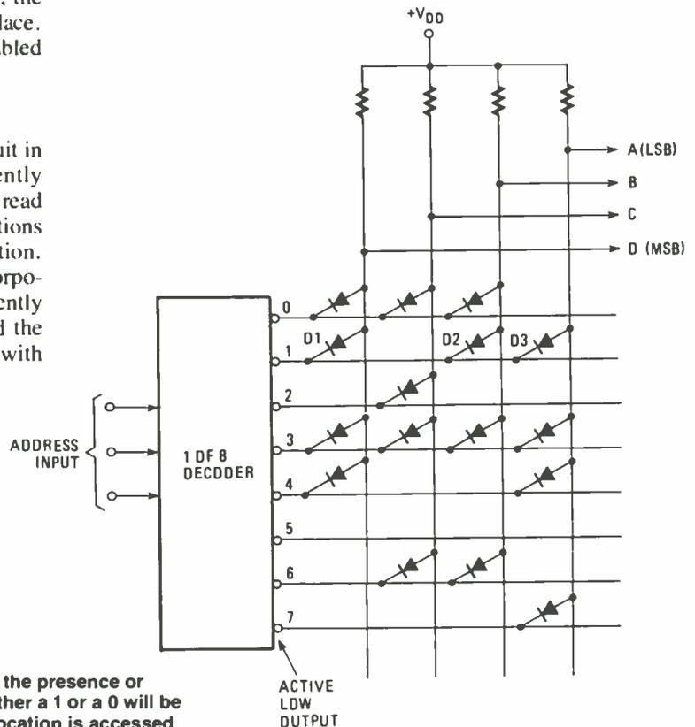
**Fig. 9—In this illustration of a ROM, the presence or absence of a diode determines whether a 1 or a 0 will be sensed when a particular memory location is accessed.**
