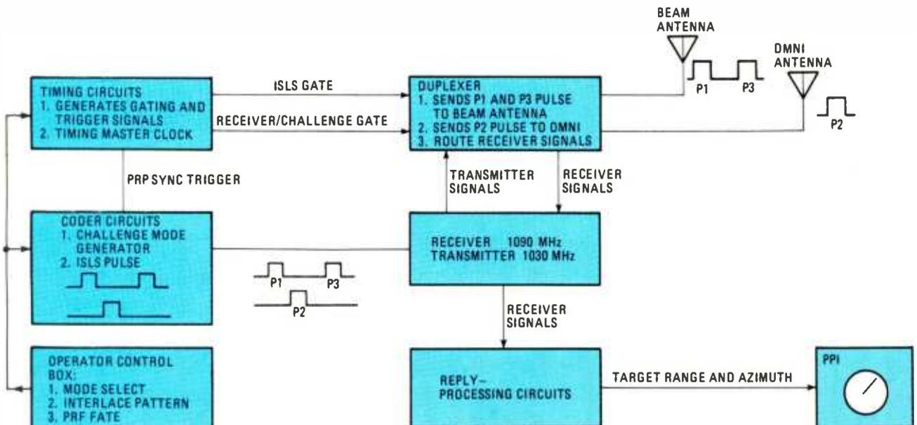
Fig. 2—The interrogator system is a complex conglomeration of several subsystems designed to interact with each other. The subcircuits, in conjunction with two antennas, transmit challenges to and process replies from the target craft.
