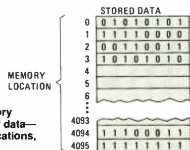
Fig. 1—This illustration of the organization of a memory chip—which is capable of storing 4K or 4096 bytes of data—shows that the chip is made up of several storage locations, each having its own distinct address (0–4095).
