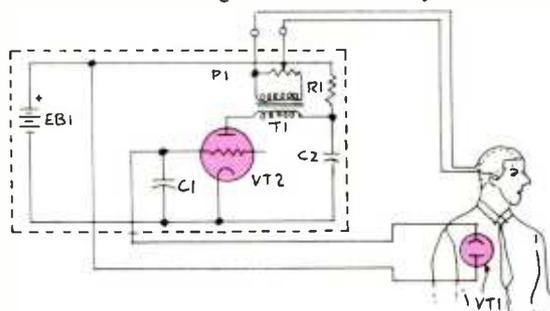
**Fig. 2—**This illustration shows a system, for which J.D. Shaw was issued a patent in 1955; it was specifically designed for informing the blind of ambient light levels.
