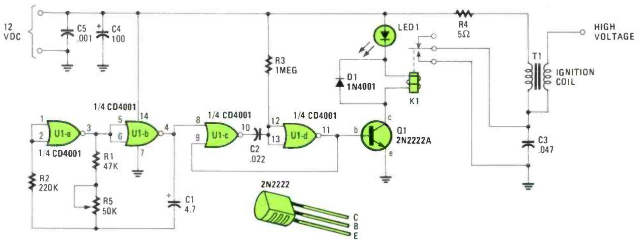
Fig. 1—The Fence Charger, for the most part, consists of a handful of easily obtainable parts. The coil, however, comes from the standard ignition system of 1960-era GMC cars. Capacitor C3 is the original component used in the system.
