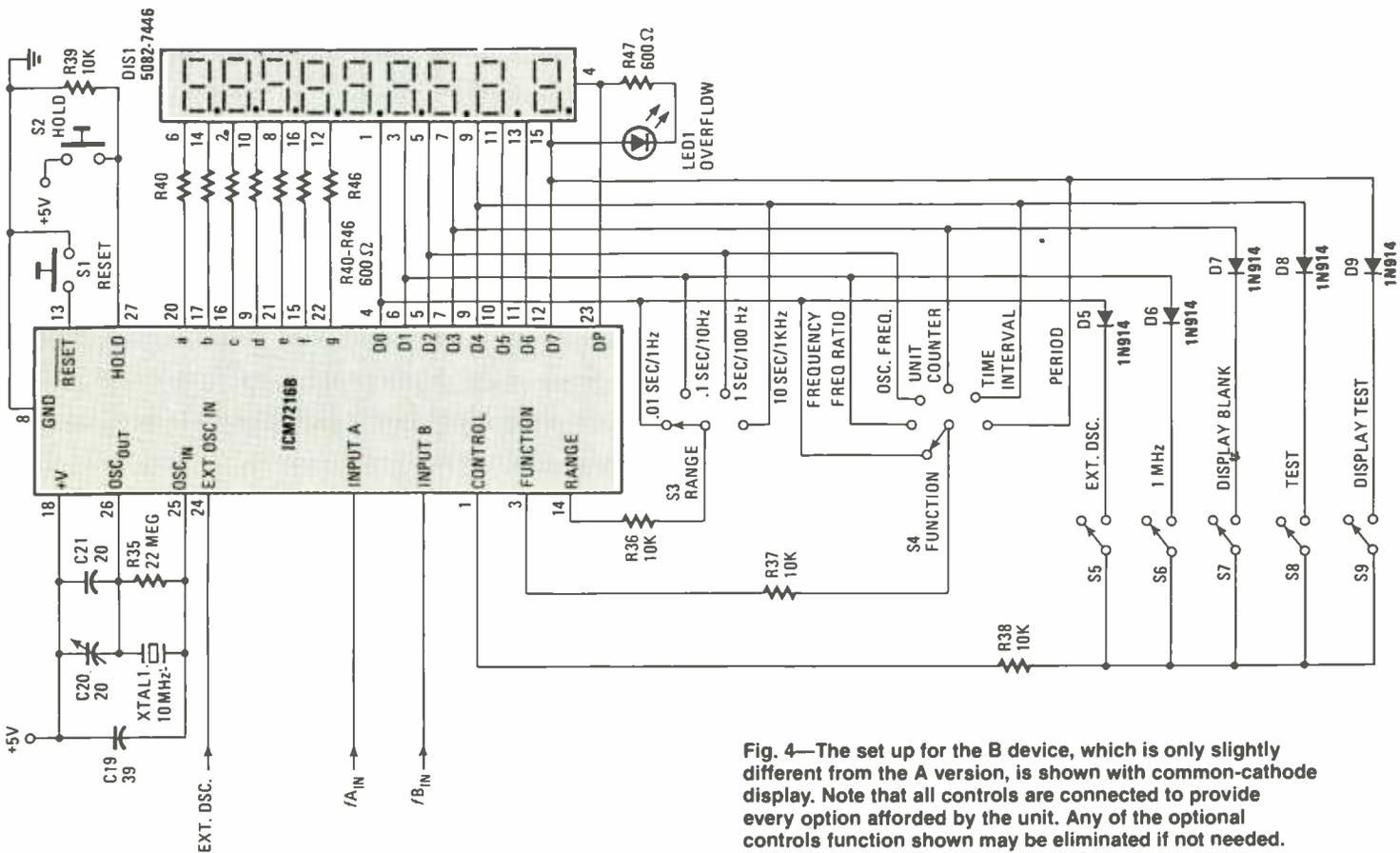
Fig. 4—The set up for the B device, which is only slightly different from the A version, is shown with common-cathode display. Note that all controls are connected to provide every option afforded by the unit. Any of the optional controls function shown may be eliminated if not needed.
