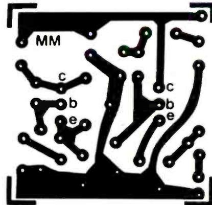
Fig. 2—The full-scale foil pattern shown may be lifted from the page and used to etch the printed-circuit board for the Magnetometer.
