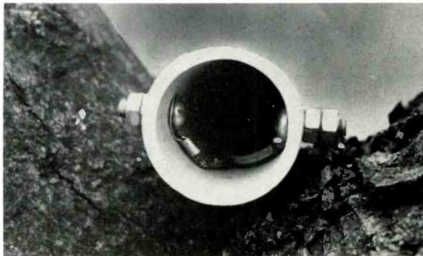
This view of the top of the PVC piping shows that the coax cable terminates in large ring tongues, which are then secured to the mast using nuts and bolts. The antenna wires are then connected to the bolts.
