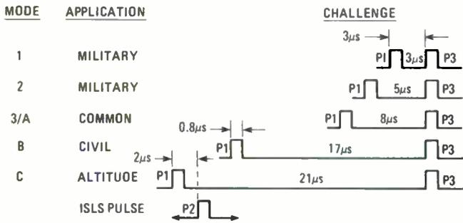
**Fig. 3**—This diagram gives the challenge modes generated by the coder circuits of the interrogator system, along with the uses for that mode. The mode of the transmission is determined by the time lapse between the leading edges of the P1 and P3 framing pulses. For instance, if the framing pulses are separated by 8  $\mu$ s, the transmission is mode 3/A, which is common to both civil and military use.
