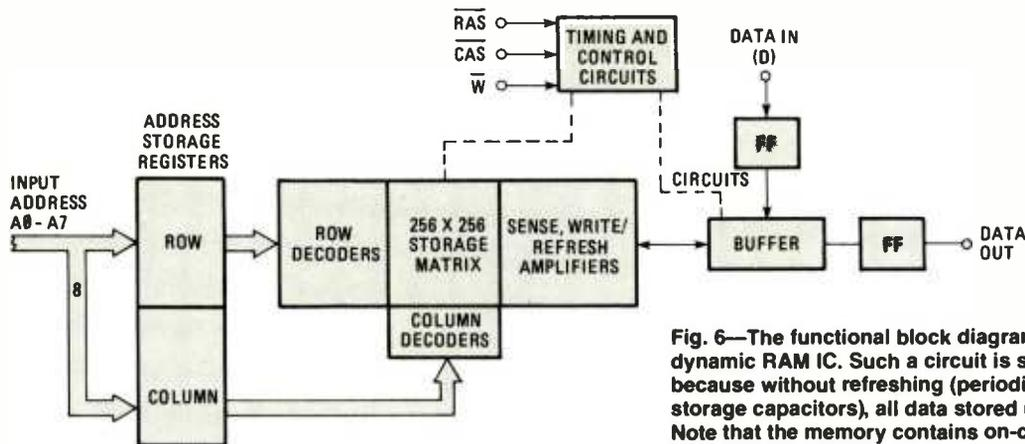
Fig. 6—The functional block diagram of a 4164,  $64\text{K} \times 1$  dynamic RAM IC. Such a circuit is said to be volatile because without refreshing (periodically recharging of the storage capacitors), all data stored in memory would be lost. Note that the memory contains on-chip refresh circuitry.
