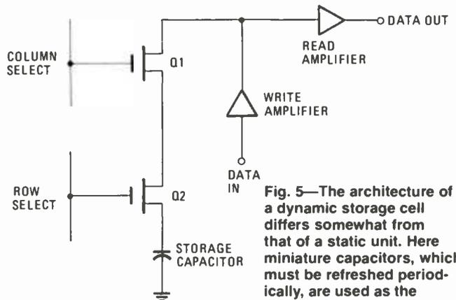
**Fig. 5—The architecture of a dynamic storage cell differs somewhat from that of a static unit. Here miniature capacitors, which must be refreshed periodically, are used as the storage elements.**
