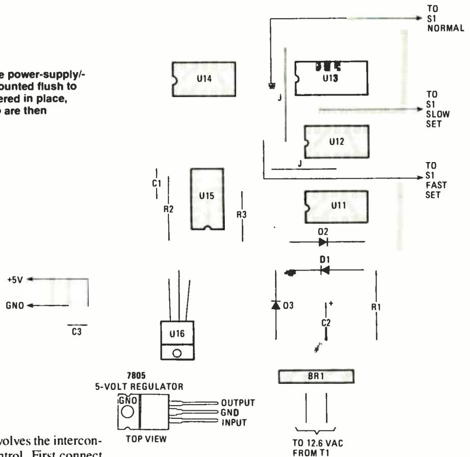
to SLOW to check for proper sequence of numbers. Check for proper timing by setting S1 to FAST; that should advance the display at a rate of 1 hour per second. (There should be 60 Hz at the FAST mode tap). In the SLOW mode, the display advances at rate of 1 minute per second (1 Hz). And in the NORMAL mode, the display's progression is at a rate of 1 count per minute (a frequency of 0.0167 Hz).
