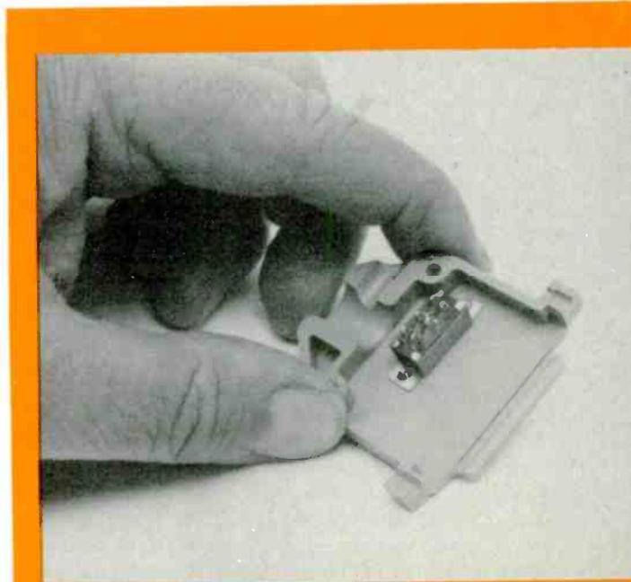
Install a subminiature DPDT slide switch on one half of a D-connector's plastic hood. Be sure to allow for cable leads to fit around switch. Refer to the text.
