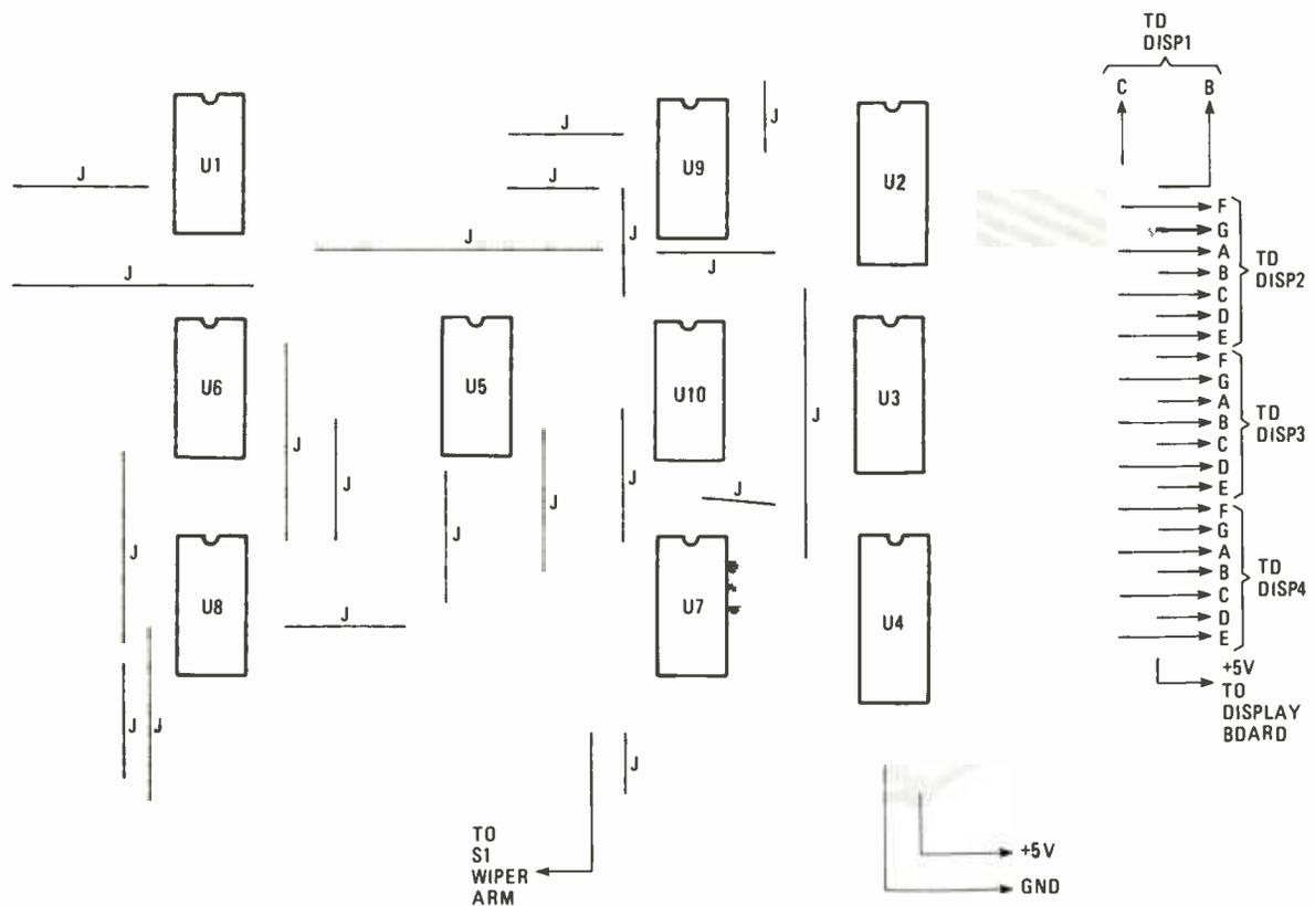
Fig. 10—The parts-placement diagram for the counter/display driver board. A 34-conductor ribbon cable is used for connections between this board and the display board, although only 24 are actually used. The parts are placed on the circuit board in about the same position as shown in the schematic diagram, Fig. 2. Align the pins of each chip with its appropriate socket and be sure that those tiny wonders are properly seated, and make sure that no pins bend under the chip.
