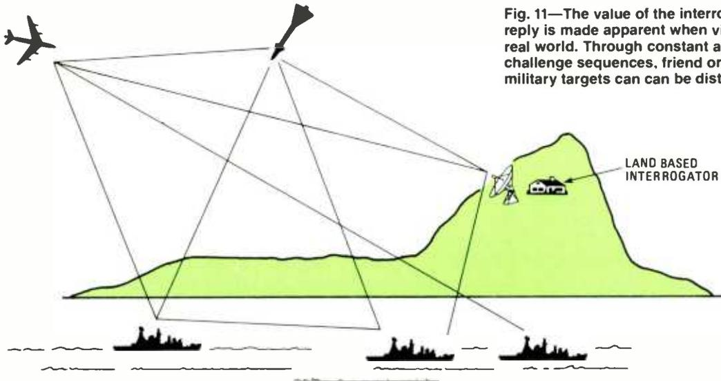
Fig. 11—The value of the interrogator's challenge and reply is made apparent when viewed in the context of the real world. Through constant and repeated reply and challenge sequences, friend or foe, civil, commercial, or military targets can be distinguished from each other.
