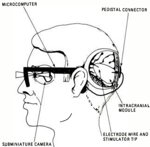
**Fig. 1—**In the Dobbelle device of the future, a glass eye, containing a subminiature camera, might be surgically implanted in the orbit and attached to the eye muscles. An intracranial module embedded in the visual control center of the brain would receive signals (based on the input from the camera) via a micro-miniature computer contained in ordinary eyeglasses, thereby, stimulating the visual center, giving rise to the sensation of sight.
