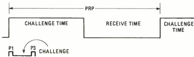
**Fig. 4**—The pulse repetition period, as shown, is the time between challenges, and extends from the time the challenge is issued to the end of the receiver period—which is actually the time between the leading edges of the P1 pulses in successive challenges.
