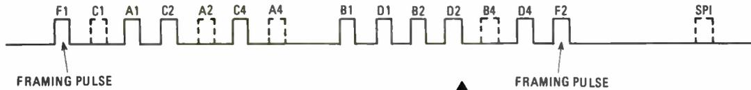
**Fig. 8**—The reply code transmission from the target craft is similar to the pulse train shown here, which is for a 1367 reply code. The coding bits shown in dashed lines are omitted from the transmission.
