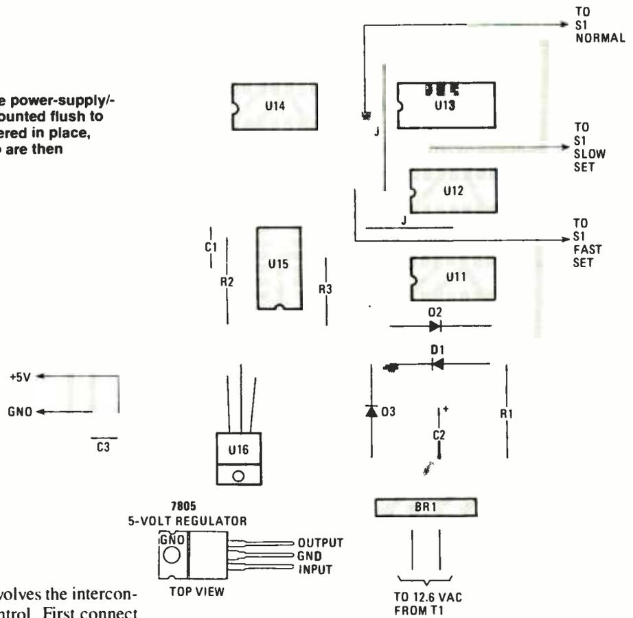
to SLOW to check for proper sequence of numbers. Check for proper timing by setting S1 to FAST; that should advance the display at a rate of 1 hour per second. (There should be 60 Hz at the FAST mode tap). In the SLOW mode, the display advances at rate of 1 minute per second (1 Hz). And in the NORMAL mode, the display's progression is at a rate of 1 count per minute (a frequency of 0.0167 Hz).
