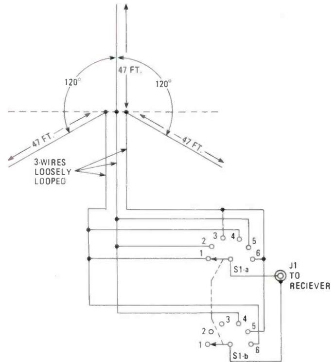
Fig. 2—The three-element Flexo installation provides greater flexibility over the two-wire type by allowing six combinations.
