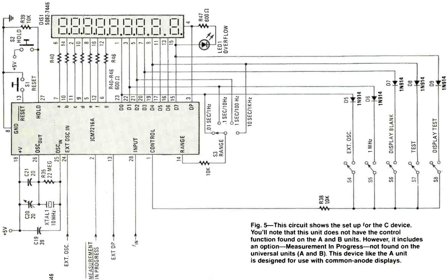
Fig. 5—This circuit shows the set up for the C device. You'll note that this unit does not have the control function found on the A and B units. However, it includes an option—Measurement In Progress—not found on the universal units (A and B). This device like the A unit is designed for use with common-anode displays.
