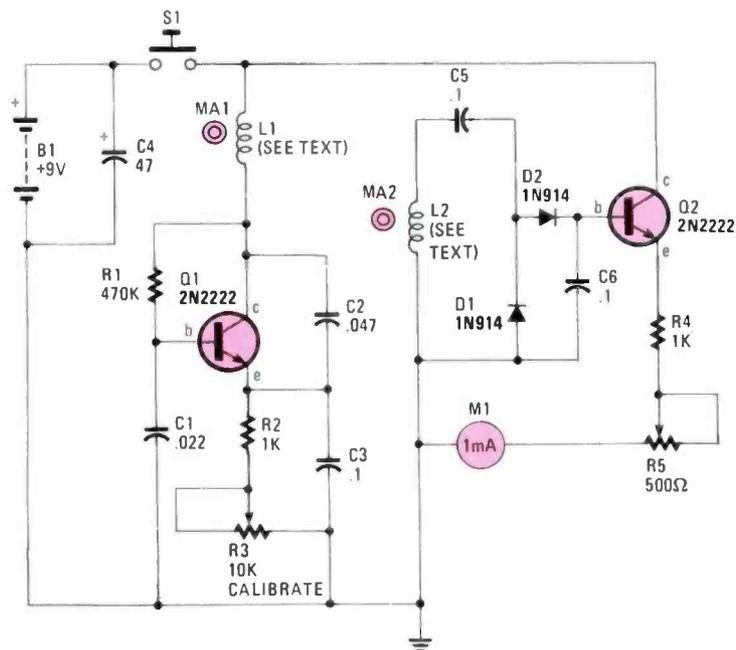
Fig. 1—In the schematic diagram of the Magnetometer note that along with the two coils, L1 and L2, there are also two magnets, MA1 and MA2. Together, those components form the sensory portion of the circuit.
