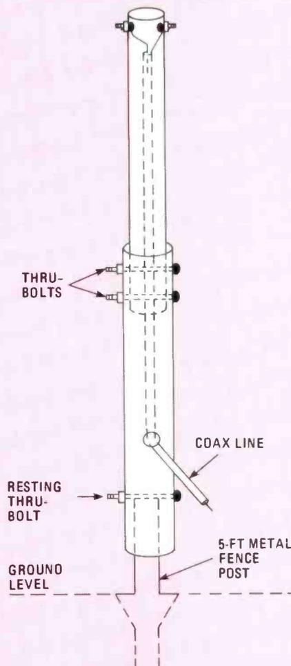
ble as needed. Connect the wires that will act as the RF pick-up element. If guys are to be used, connect them now. Use nylon stranded rope—the smallest diameter you can buy. Drop the mast over the fence post and secure with bolts. And finally, secure the guys. Taller masts can be built by using longer or additional lengths of PVC tubing.
