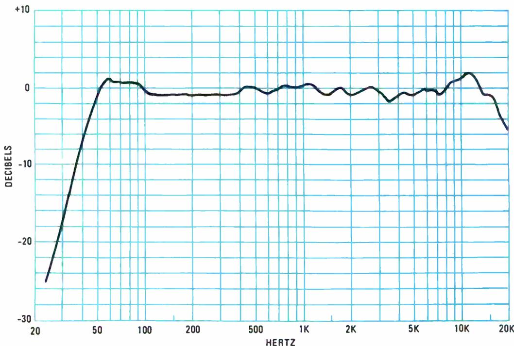
Fig.5—The frequency-response curve of a full-scale domestic loudspeaker system using Philips drivers and a Philips-designed, sealed enclosure. It could readily cope with low-end bass boost.
