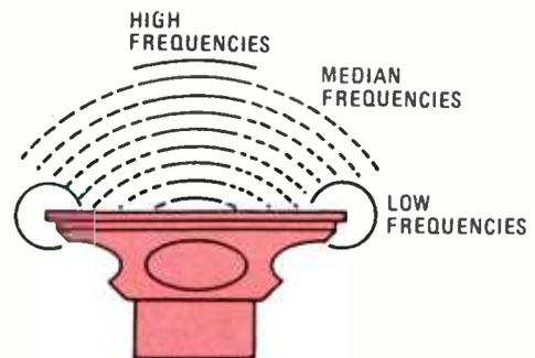
**Fig. 1—The sound-propagation pattern for an unmounted full-range loudspeaker. Baffling is necessary to prevent low-frequency energy from being merely pumped back and forth around the edge of the housing.**
