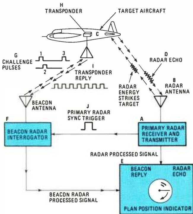
Fig. 1—Examples of primary and beacon radar are compared. Note that in the primary radar system, the transmitted signal is reflected from the target back to the source, and displayed on the PPI as a blip to indicate the target's location; whereas, in beacon radar, a challenge signal from the interrogator is picked up by the target, which then decodes the signal and sends a reply to the interrogator.
