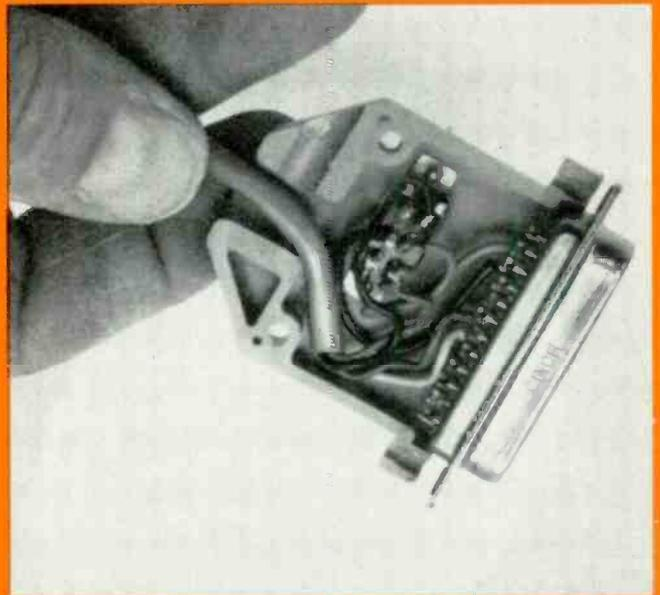
Wire the cable and switch according to Fig. 1, and carefully route the cable around the switch, so that the cable doesn't get pinched when the other half of the hood is secured.
