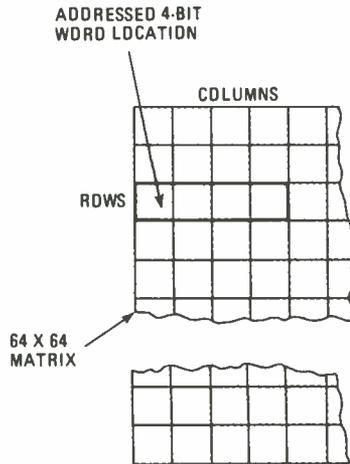
Fig. 8—The 2114, with its 1K × 4 configuration, can store 1024 4-bit words. The memory is arranged in a 64 × 64 matrix, providing 4096 individual storage cells.
