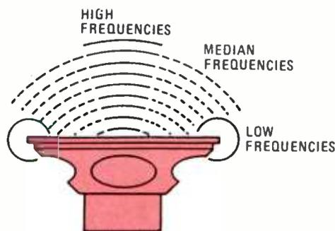
**Fig. 1—The sound-propagation pattern for an unmounted full-range loudspeaker. Baffling is necessary to prevent low-frequency energy from being merely pumped back and forth around the edge of the housing.**
