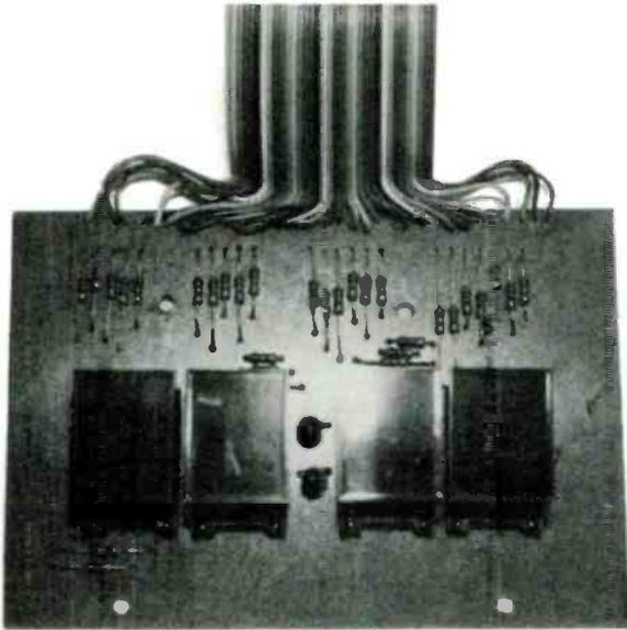
A 34-conductor ribbon cable is used to connect the display board to the counter/display driver board. Also, note that the seven-segment display modules are mounted in 28-pin sockets. The bottom socket contacts protruding from beneath the displays are used as test points. If at any point along that line, you are unable to get a 5-volt reading, check to make sure that power is being delivered to the board. Also check the copper traces for breaks.
