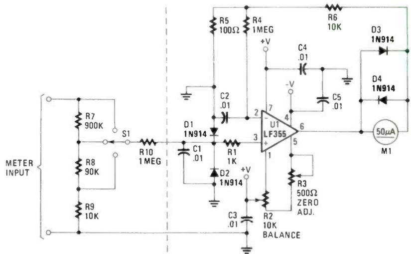
Fig. 4—This analog millivoltmeter, using the LF355 JFET op-amp, can be put together for just a few bucks. And the three-step attenuator network, consisting of R7-R9, can be expanded for greater range and versatility.
