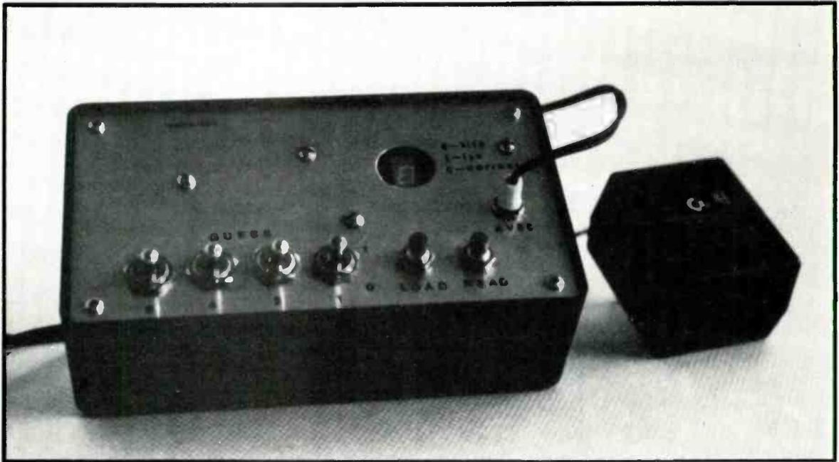
the count reaches 15, U2 then recycles to 0 and starts over again. Since U1 puts out about 1000 pulses per second (1 kHz), you have no way of knowing what number is loaded into U2 when S1 is released. U2 translates the count into a 4-bit binary number, which is then fed to U3, a 4-bit magnitude comparator. The comparator determines whether or not its two inputs are equal, or if one signal is greater than or less than the other signal.
