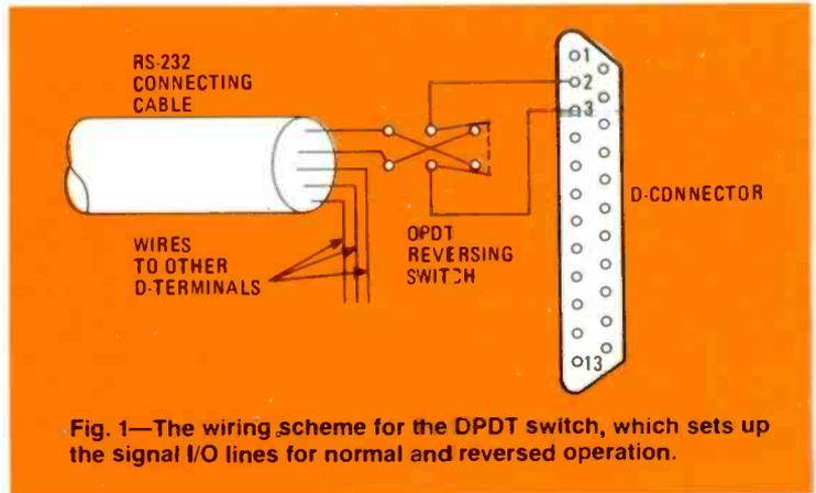
Fig. 1—The wiring scheme for the DPDT switch, which sets up the signal I/O lines for normal and reversed operation.
