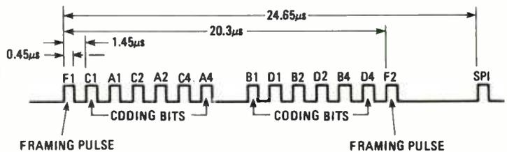
**Fig. 6**—After the reception of the interrogator's challenge transmission, the target craft's reply is characterized by a 12-bit code sandwiched between two framing pulses, F1 and F2.
