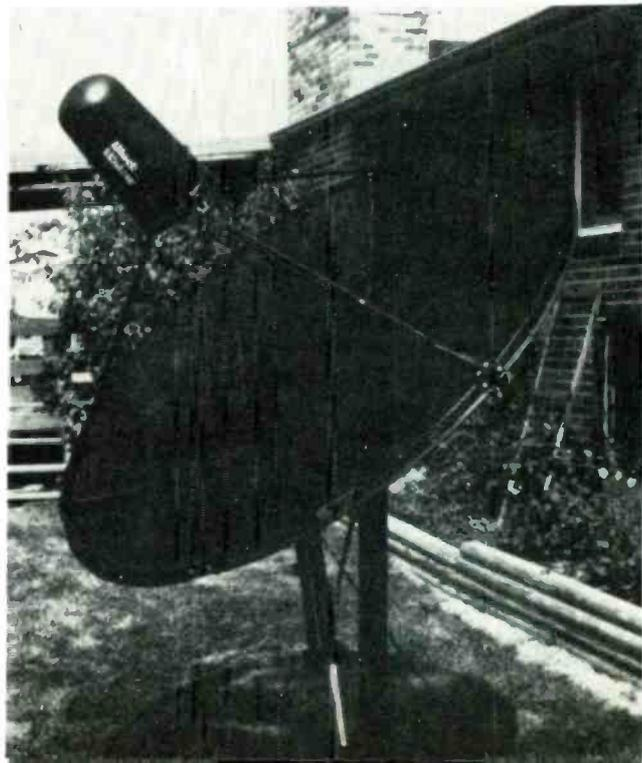
The six-foot dish of the Series II is secured to a polar mount. As the antenna is rotated on its polar axis, the dish scans the available satellites viewable from your locale.
