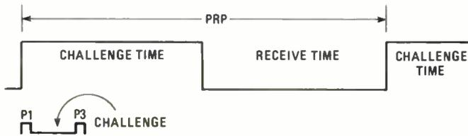
**Fig. 4**—The pulse repetition period, as shown, is the time between challenges, and extends from the time the challenge is issued to the end of the receiver period—which is actually the time between the leading edges of the P1 pulses in successive challenges.
