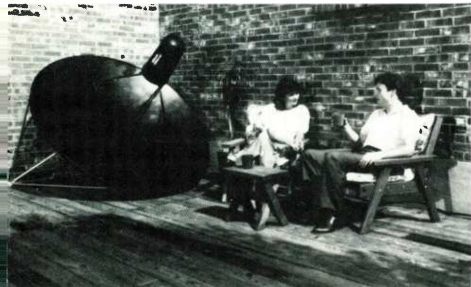
Regardless of whether you're interested in a basic or deluxe model, each system consists, essentially, of the same components: the parabolic dish (also called the antenna), LNA, and receiver (see photos). The dish, like any other antenna, is a signal gathering device, which is pointed toward the sky at an angle dependent on the site's location in relationship to the orbiting *birds*.
