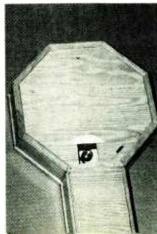
Every digital clock has a time-setting switch. The knob for S1 can be seen at the rear of the clock. Four positions provide a time-holding feature, a slow set where the time advances slowly, a fast set when the time advances rapidly, and a normal running position once the correct time has been achieved.
