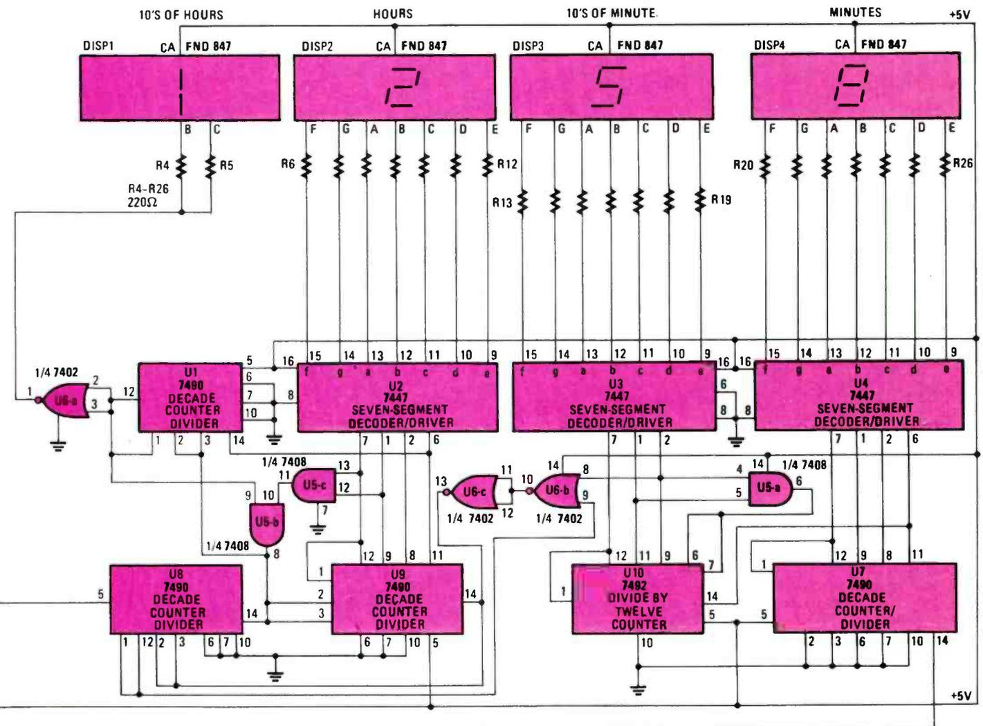
Fig. 2—Schematic diagram of the entire TTL Clock. The circuit consists of three separate sections: The display, the counter/display driver, and the power supply/frequency divider. The three sections are laid out on individual printed-circuit boards.
