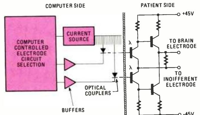
Fig. 5—The Dobelle device using monopolar, biphasic stimulation: A small electrode is applied to the cortical tissue, while a large indifferent electrode, placed under the scalp, is used for the return current.
