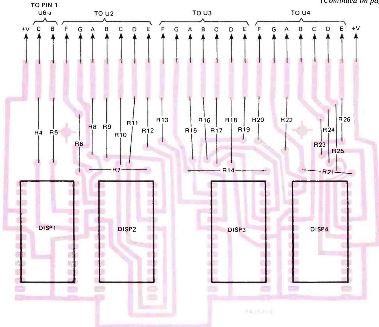
Fig. 8—The parts layout for the display board shows that only the segments used for DISP1 are to be connected. Unused pins of the socket are connected to +5V for use as test points. One of the +V tie-points, which are located on either side of the printed-circuit board, is used for future circuit additions; for instance, chimes might be added.
