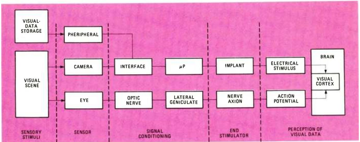
Fig. 3—A comparison between physiologically and artificially induced sight. Note the relationship between the various parts of the artificial vision system and its natural counterpart.
