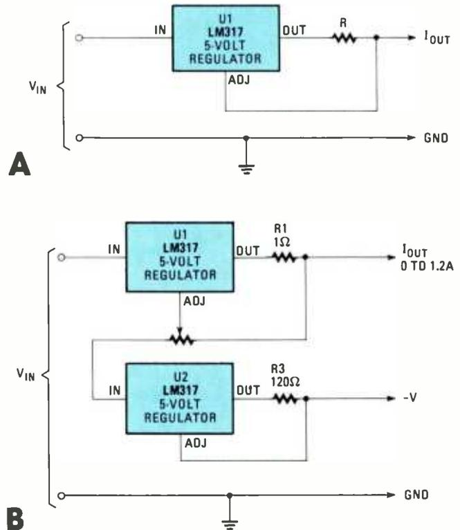
Fig. 3—Both the basic (A) and an extended version (B) of the constant-current setup is shown built around the LM317 positive, adjustable regulator. By using the LM317, most of the problems associated with using three-terminal regulators in constant-current applications can be eliminated.
