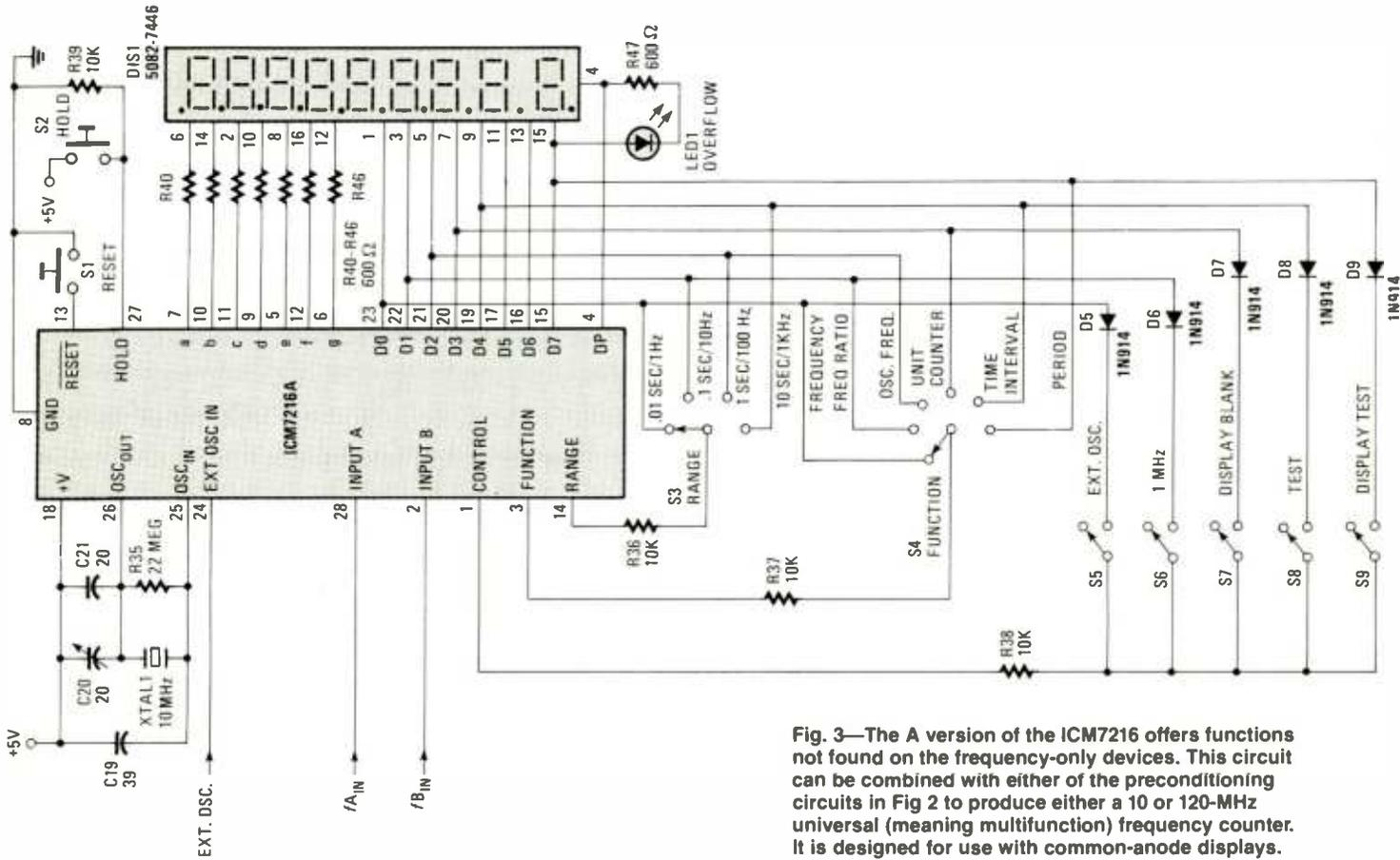
Fig. 3—The A version of the ICM7216 offers functions not found on the frequency-only devices. This circuit can be combined with either of the preconditioning circuits in Fig 2 to produce either a 10 or 120-MHz universal (meaning multifunction) frequency counter. It is designed for use with common-anode displays.
