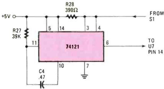
Fig. 4—This circuit, made from an additional 74121 monostable multivibrator and three external components, can be placed between switch S1 and the pin 14 input of U7, to eliminate false counting that may occur because of a noisy (bouncing) switch.
