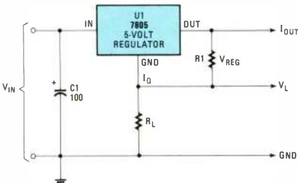
Fig. 1—A circuit capable of a constant-current output can be built from three-terminal regulators, such as the LM309, 7805, etc.
