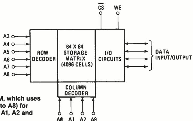
Fig. 7—Block diagram of the 2114 4K-bit RAM, which uses a 10-bit address code; six address lines (A3 to A8) for the row decoder and four address lines (A0, A1, A2 and A9) for the column decoder.
