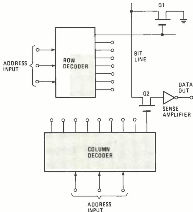
Fig. 10—In this simplified diagram of one type of ROM structure, the presence or absence of a MOSFET transistor (in this example, Q1) at each possible junction determines whether 1 or 0 is stored. If a MOSFET exist (meaning, is connected) at the junction, a binary 1 is stored, but if not, a binary 0 is stored.
