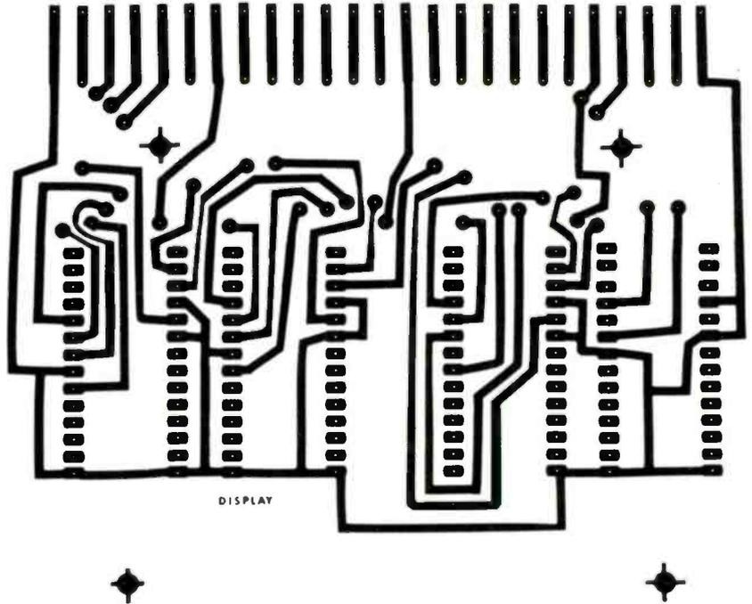
Fig. 6—Foil pattern of the power supply/frequency divider board. When mounting the diodes and electrolytic capacitor, be careful of their orientation.
