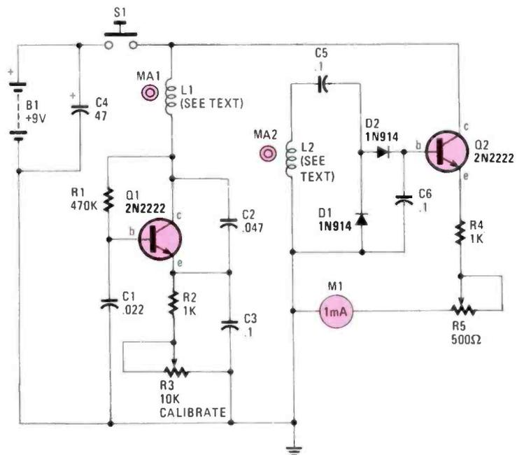
Fig. 1—In the schematic diagram of the Magnetometer note that along with the two coils, L1 and L2, there are also two magnets, MA1 and MA2. Together, those components form the sensory portion of the circuit.
