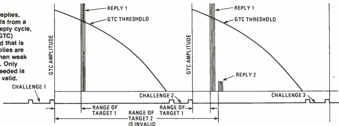
challenge 1 and is within radar range. Thus, the reply pulse amplitude is greater than the GTC threshold. But, REPLY 2 is invalid since it's a target's reply from challenge 1 and is outside the radar's range. The reply pulse amplitude, therefore, is less than the GTC threshold.
