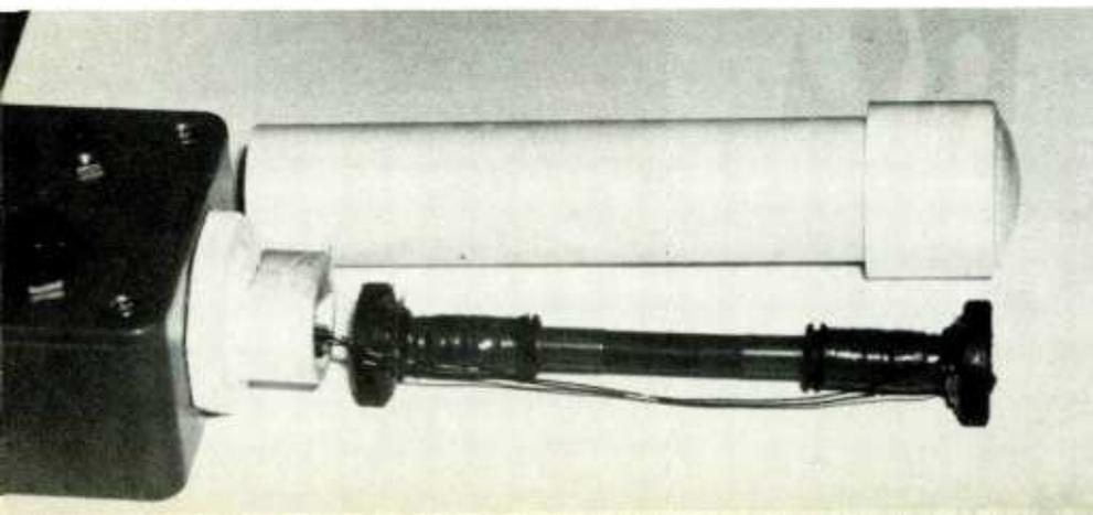
The Magnetometer's housing is outfitted with a plastic pipe plug through which the probe and the printed circuit are connected. Once connected, the probe is placed inside its PVC housing and covered with a plastic pipe cap. Then the probe assembly is affixed to the project box by pushing the PVC tubing over the plastic pipe cap.
