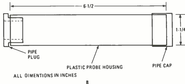
**Fig. 4—The sensor probe is fabricated using the specified parts (see text for details). Grommets can be glued in place on the ferrite rod to act as a border when winding the coils.**
