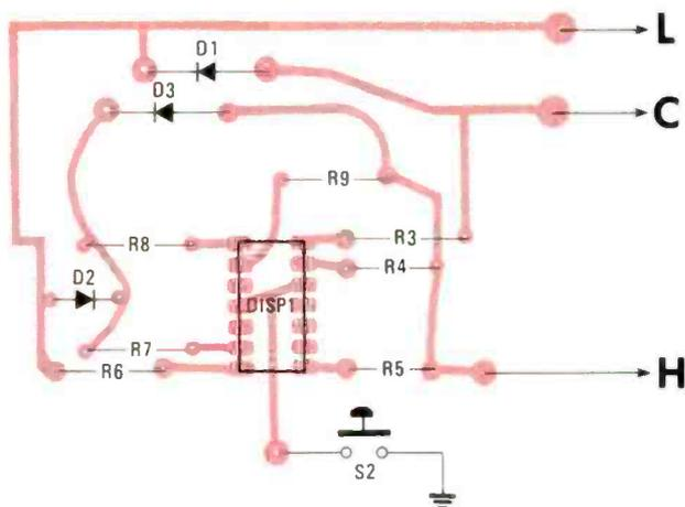
Refer to Fig. 4 and Fig. 5, the parts layout for the main circuit and display boards, respectively. Begin by installing the passive components, resistors and capacitors, first; then move on to the semiconductors, populating one board at a time.
