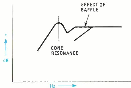
Fig. 4—Fitting a loudspeaker to a baffle pushes the 6dB/octave roll-off further down in the range. The cone resonance can become very prominent, as a result, if it's not sufficiently damped by the associated amplifier.
