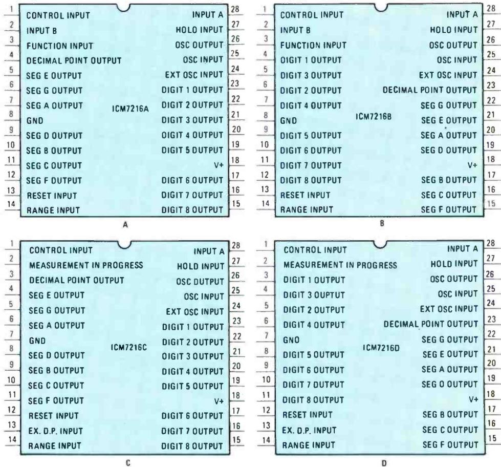
Fig. 1—The ICM7216, available in four “flavors” (A, B, C, and D), is a fully integrated 10-MHz counter that has on board all the necessary circuitry to build either a universal or frequency-only counter. The A and B units are universal counters, while C and D devices function as frequency-only counters. The A and C units are designed for use with 7-segment, common-anode, light-emitting diode displays; while, B and D suffix devices are compatible with common-cathode displays.
