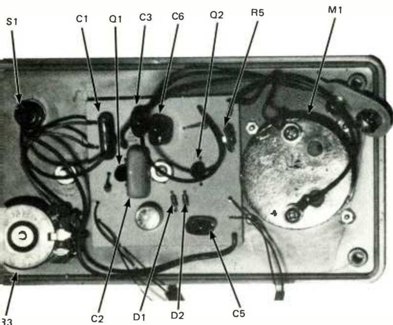
**A view inside the Magnetometer project pinpointing the printed-circuit board and major circuit components.**
