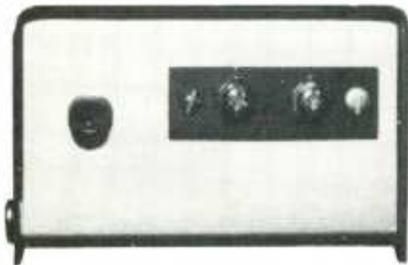
The switch box is simply an inexpensive metal cabinet that houses the selector switch, with the switch positions labeled on the front. On the rear of the cabinet, two screw-type terminals are mounted to which the feed line is attached. A shielded phono jack is also provided as the receiver connection.
