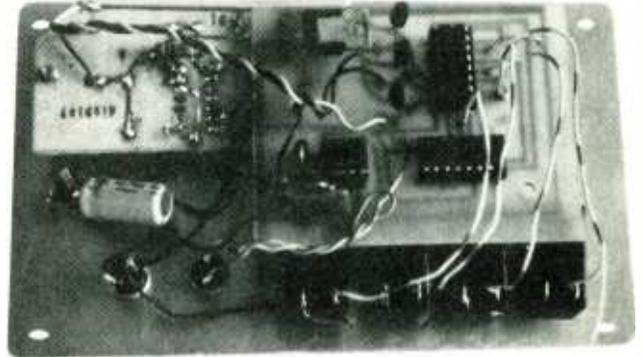
The Super ESP Tester is built on two small printed-circuit boards to allow them to be easily mounted to the back of the front panel of the project box. Note that a large electrolytic capacitor (C2) is mounted on the panel as well.
