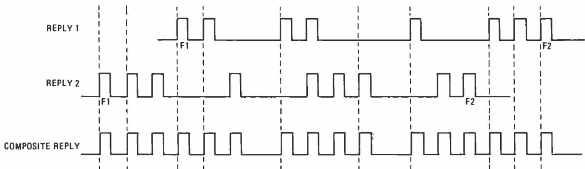
Fig. 12—Garbling is an example of what can happen when two aircraft are separated in altitude by only a few hundred feet, while being equal distances from the airport. The reply signals from the two craft are interlaced, producing a composite of the two replies.
