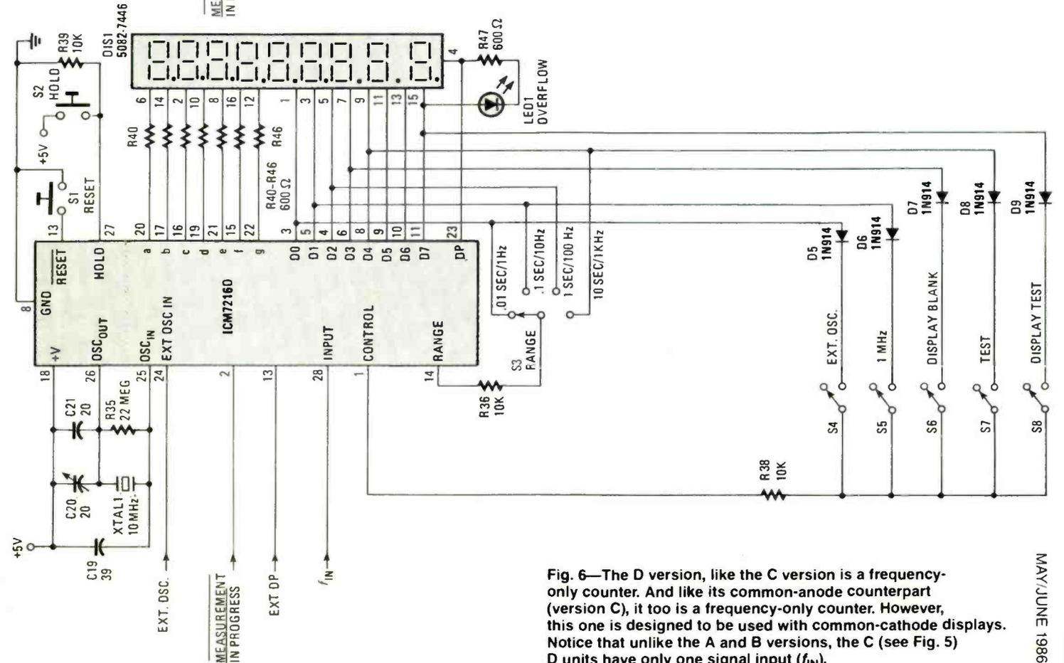
Fig. 6—The D version, like the C version is a frequency-only counter. And like its common-anode counterpart (version C), it too is a frequency-only counter. However, this one is designed to be used with common-cathode displays. Notice that unlike the A and B versions, the C (see Fig. 5) D units have only one signal input (f<sub>IN</sub>).
