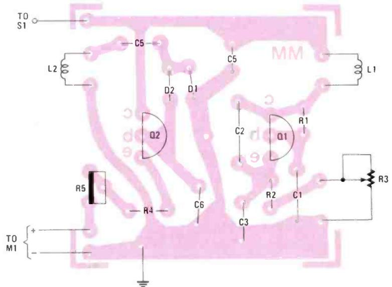
Fig. 3—An x-ray view of the printed-circuit board showing the parts layout for the Magnetometer. Coils L1 and L2 are shown as if mounted in the printed-circuit board, but they are not. Instead, they are wound around the ferrite rod and attached to the printed circuit.
