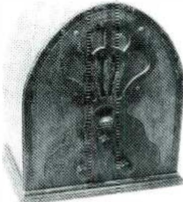
The Balkeit Model 55 typifies the downsized AC sets made possible by more efficient tubes and more powerful radio stations. Its "gothic cathedral" case houses a 5-tube (with rectifier) circuit.
