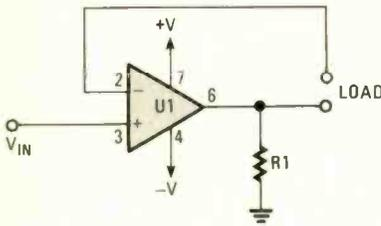
**Fig. 7—The non-inverting V-to-C converter is almost identical to the inverting version shown in Fig. 6, other than a simple modification.**
