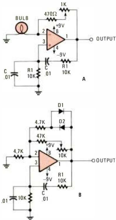
**Fig. 17**—If you can't get the light bulb needed for the circuit in A, then you can use the circuit in B. Its output will not be as clean, but is good enough here.
