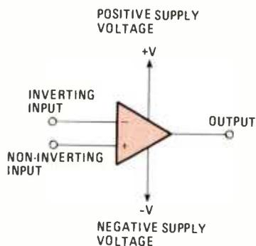
Fig. 2—The power-supply connections will not be shown in the diagrams after this one. You will assume they are used as shown here. Note that neither goes to ground.
