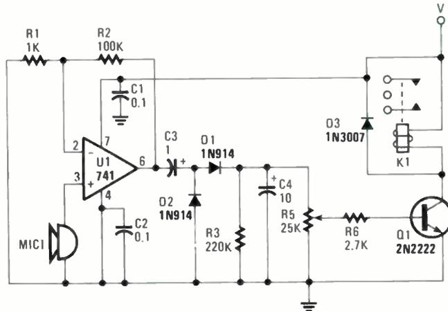
**Fig. 3—The op-amp output at pin 6 is rectified by diodes D1 and D2, filtered by capacitors C3 and C4. The resulting DC output is applied to the base of transistor Q1, turning it Q1 on and, thus, the relay, activating the load.**
