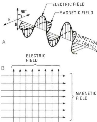
Fig. 1—Radio and TV waves are electromagnetic (EM) waves exactly like light, infrared, and ultraviolet, consisting of two mutually perpendicular oscillating fields (electric and magnetic, shown in "A"). If (as shown in "B"), at a great distance from the center, we take a look at a small slice of the advancing wavefront, we would be able to observe the electric and magnetic field vectors at right angles to each other.
