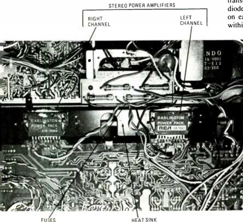
**Critical voltages on the suspected power IC may indicate a leaky IC component or unbalanced DC circuit. Interchange the two output IC components in both channels to see if it is defective when you do not have a replacement on hand.**
