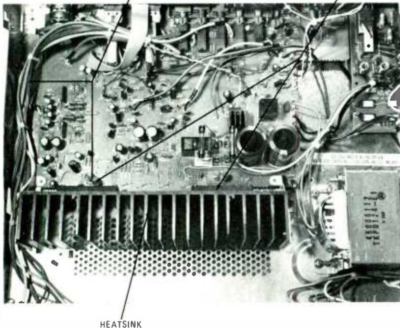
**Transistors may be checked in seconds with the diode/transistor test of the DMM. During replacement, put silicone grease on the tabs of transistors or IC's.**
