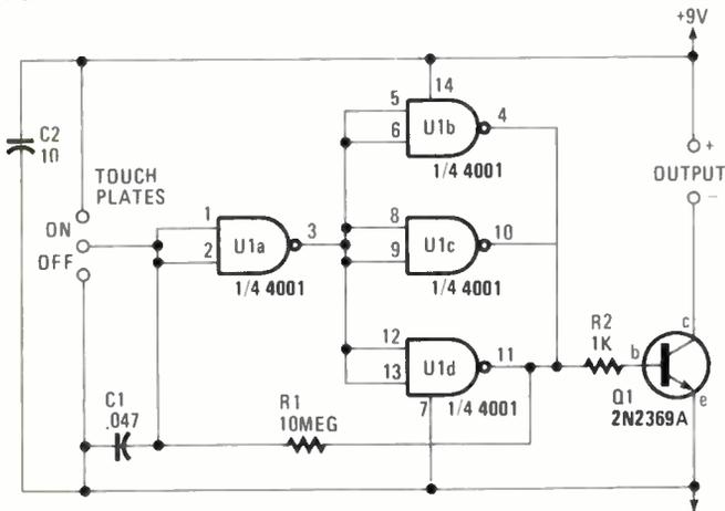
**Fig. 2—This Touch Switch (which will control 9-volt DC loads of up to 100mA) is built around a 4001 quad NOR gate. U1b to U1d along with U1a form a bistable multivibrator. Touching the two upper contacts causes Q1 to conduct, pulling its collector low; thereby, completing a path to ground through the load circuit.**
