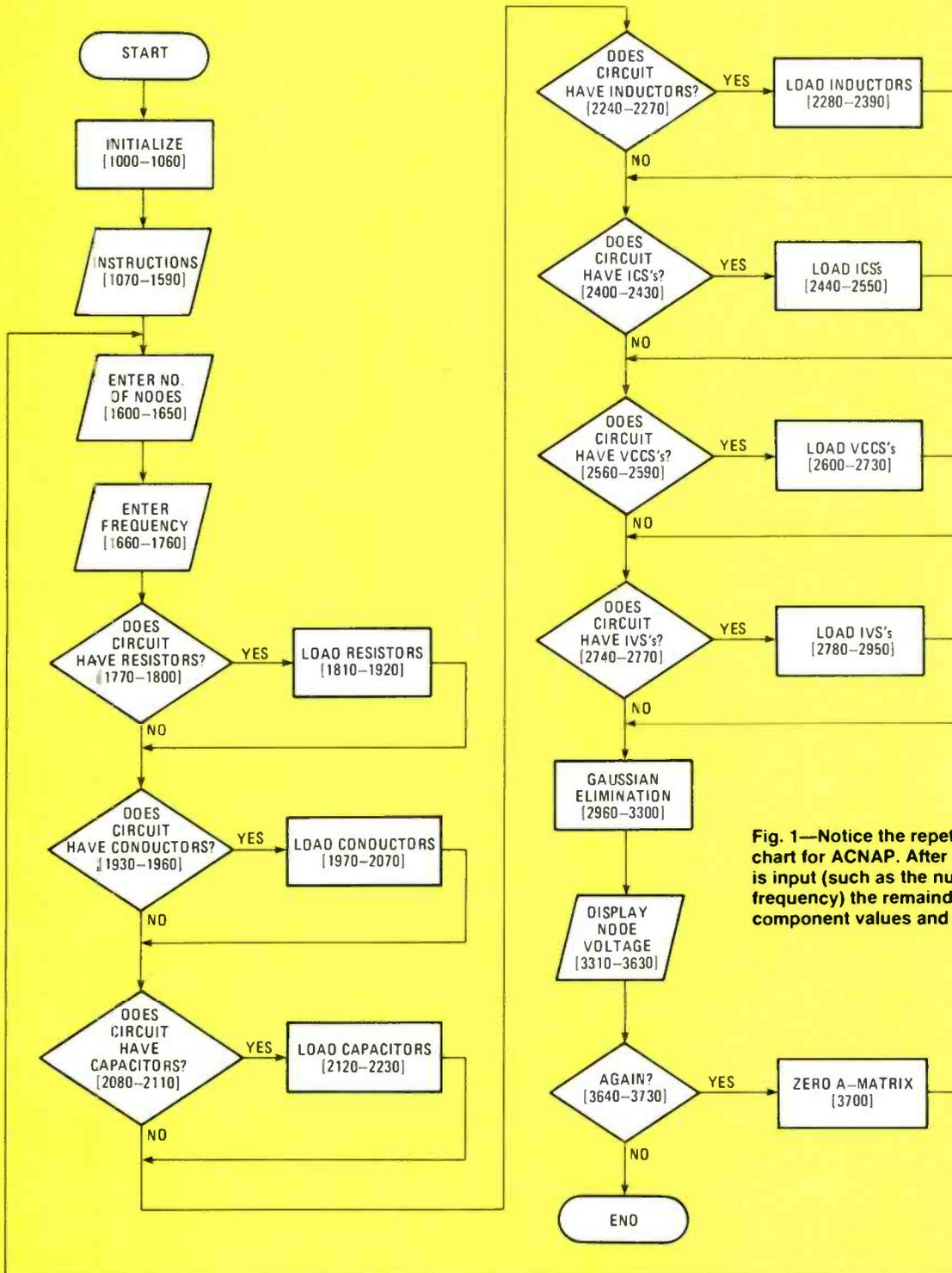
Fig. 1—Notice the repetitive nature of this flowchart for ACNAP. After main data for the circuit is input (such as the number of nodes and the frequency) the remainder of the program accepts component values and performs algebra.
