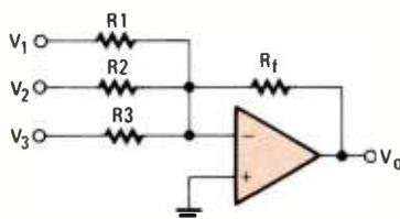
**Fig. 7—Signals can be added together using this simple summing circuit. The circuit will not only mix signals, but amplify them as well. That is useful for multi-track audio.**
