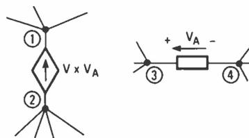
Fig. 6—When analyzing the nodes connected to a voltage-dependent current source (nodes 1 and 2) the nodes it's dependent on (nodes 3 and 4) must be solved for first.
