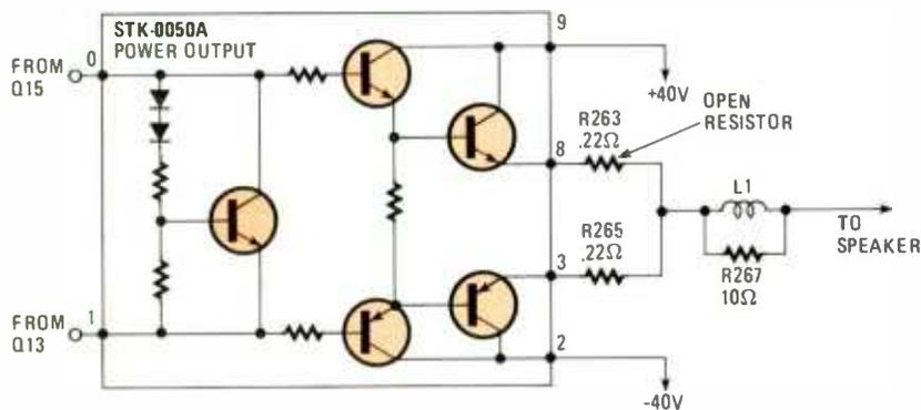
**Fig. 5—Check the base/emitter-bias circuits for open or burned resistors in the power output (IC and transistors) section of the amplifier when the output audio is weak and distorted. The open-resistor (R263 shown here) in the power output circuit (from a Pioneer model SX-780) caused excessive distortion.**
