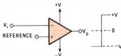
**Fig. 9—A comparator is nothing more than an op-amp with its gain wide open. Since it has no feedback resistor the output swings between the power-supply voltages.**
