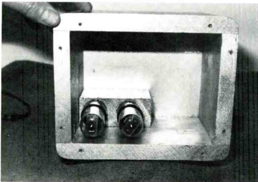
The tubes are dummies in the author's model. If you wish, you can power up the tubes using a filament transformer and nothing else. The tubes will add color and heat like the old sets.
