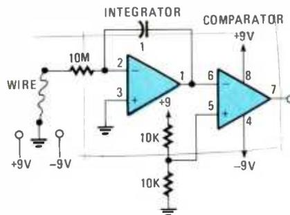
**Fig. 14—Connecting the comparator and integrator circuits causes the comparator to switch states when the integrator has been operating for a certain time and reaches 4.5 volts.**
