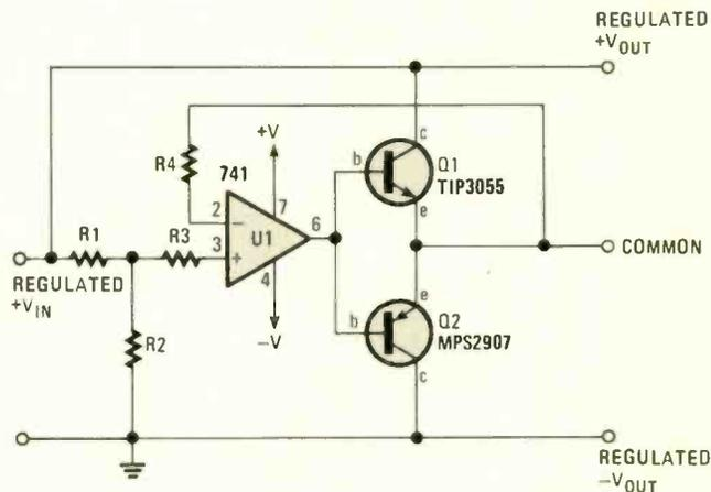
Fig. 9—The polarity splitter allows a single-ended power supply to be used as a dual-polarity power supply, with an artificial (floating) output ground. The artificial ground should never be shorted to true ground to prevent serious shock hazard and certainly damage to semiconductors.
