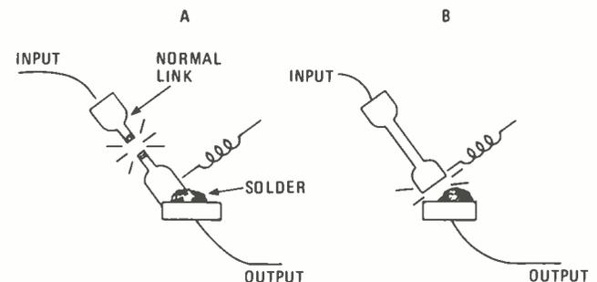
Fig. 5—A dual-action, slow-blow fuse blows in one of two modes: either the link melts under short-circuit conditions (A), or the solder blob melts due to continuous overload.
