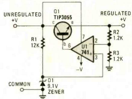
Fig. 3—Transistor Q1 is configured for series-pass operation and is controlled directly by the output of U1. The reference that's applied to the non-inverting input of U1 at pin 3 is determined by resistor R1, and zener diode D1.
