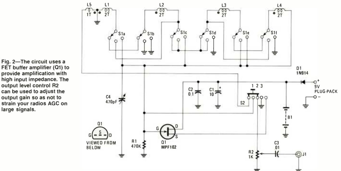
Fig. 2—The circuit uses a FET buffer amplifier (Q1) to provide amplification with high input impedance. The output level control R2 can be used to adjust the output gain so as not to strain your radios AGC on large signals.
