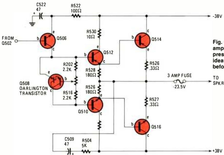
**Fig. 6—Any defective component within the DC-amplifier circuits can result in a high DC-voltage presence at the speaker terminals. It's a good idea to check the speaker terminals for DC voltage before connecting a replacement speaker.**
