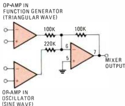
**Fig. 19**—This circuit not only adds the triangle and sine waveforms together, it amplifies one of them as well.
