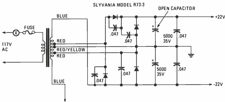
Fig. 4—Excessive hum may be caused by large filter or decoupling capacitors within the low-voltage power supply that may have opened up, or deteriorated. Hum and distortion may result from leaky output transistors or IC components.
