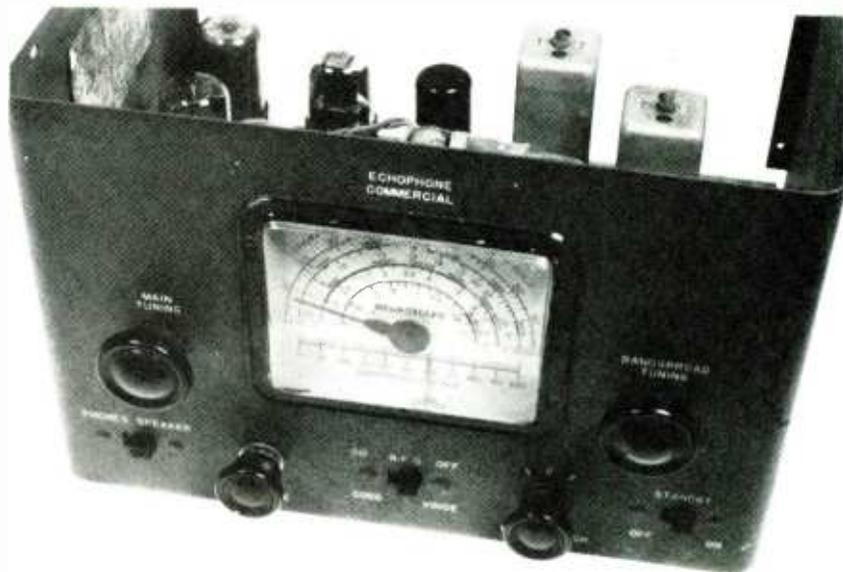
A frontal view of the reassembled Echophone. The top panel (containing the speaker) won't be replaced until the set is operating and needs no adjustment.
