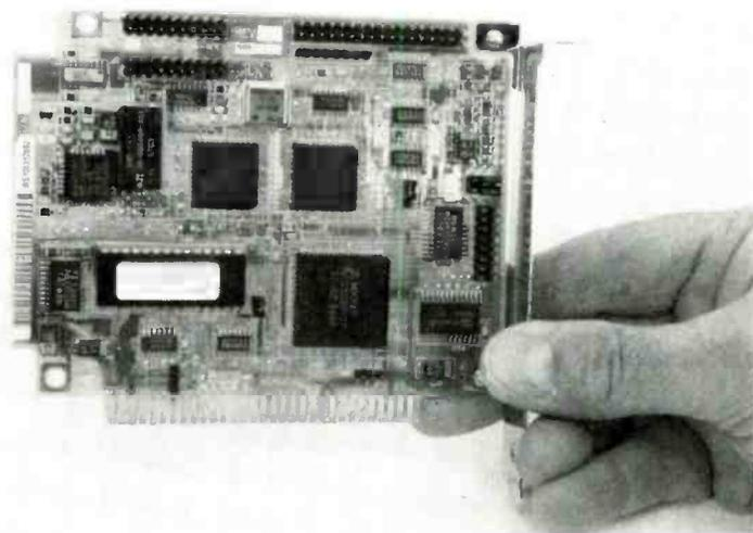
This half-size "WX-1" hard-disk controller has two smaller header terminal strips, which can each drive a disk drive. The larger header strip is split by a Y-adaptor or a two-connector cable when using two disk drives.
