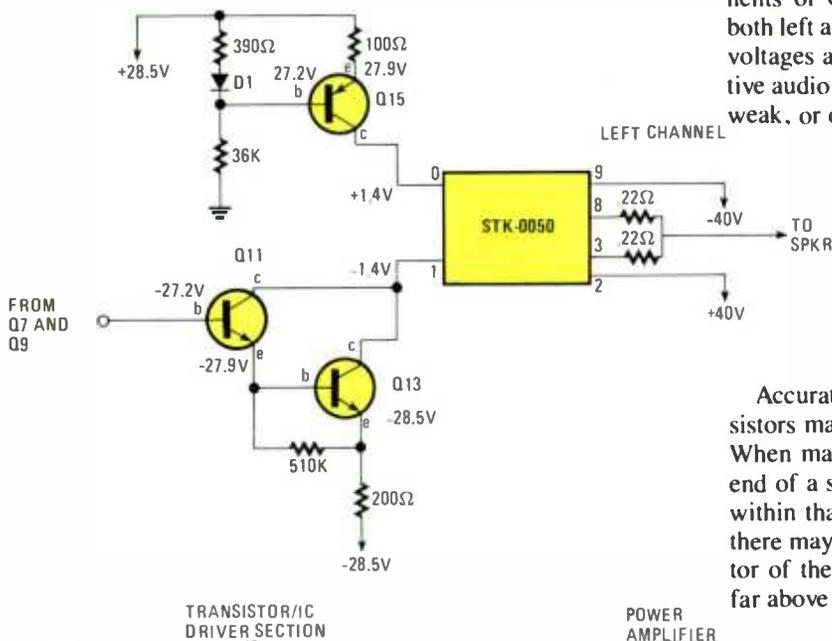
**Fig. 3—High B positive and negative voltages are found in high-powered amplifiers. Three or four voltage levels may be fed to high-powered amplifier circuits.**
