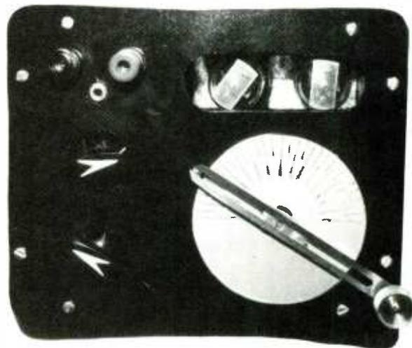
If antique knobs are not available, make some of your own. The round dial assembly was made from a piece of plastic with lines drawn through with a small soldering iron. Two coats of silver metallic spray paint makes it appear like a metal dial.
