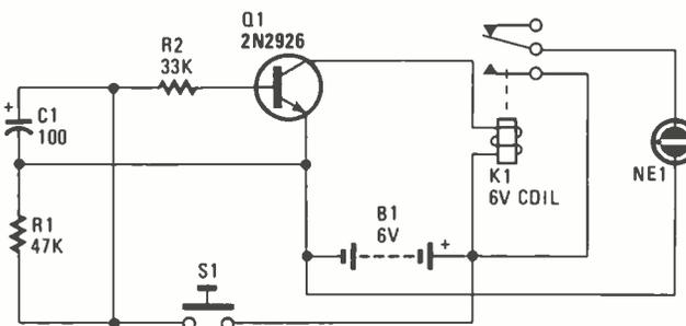
Fig. 5—Pressing switch S1, causes C1 rapidly to .7 volt, biasing Q1, which allows current to flow and operate the relay. Releasing S1 causes C1 to discharge through R2. When the charge on C1 reaches about half a volt, Q1 turns off and the relay opens.
