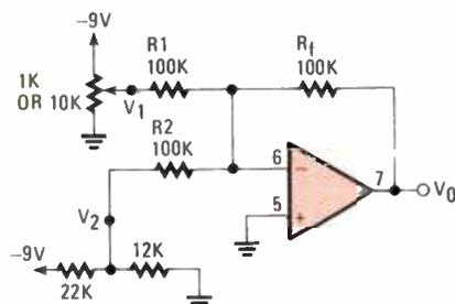
Fig. 18—This summer can actually add two voltages together as long as their sum is less than the supply voltage. The output should equal their sum since no gain is provided.
