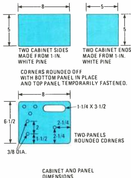
**Fig. 3—Here are the cabinet's surface dimensions. Fasten top, and side panels to the cabinet and round off the corners together with a bench or portable sander. Drill out the ends of the slotted tube areas with a 1/4-inch circle cutter.**
