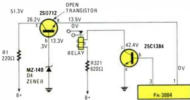
**Fig. 2—The relay malfunction may be caused by dirty contacts or an open coil winding. Check transistor and IC-controlled components when the relay itself is operating normally. Should a transistor open up, intermittent operation would result.**
