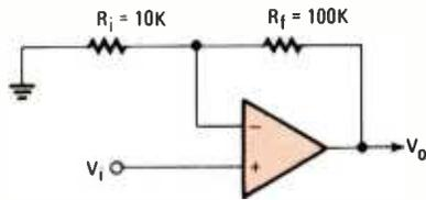
**Fig. 5—The non-inverting amplifier requires a feedback resistor at its inverting input, but it accepts input at its non-inverting input, and outputs an in-phase signal.**
