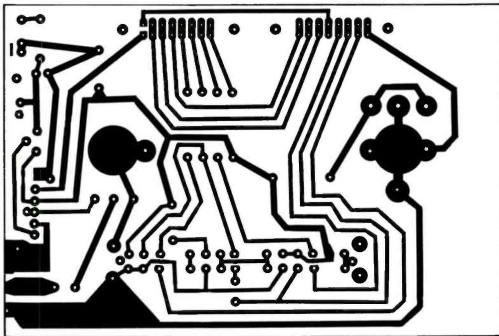
Fig. 3—The circuit-trace pattern shown here is the same size as the circuit board, so you can use this to make your own printed-circuit board using the positive resist method.
