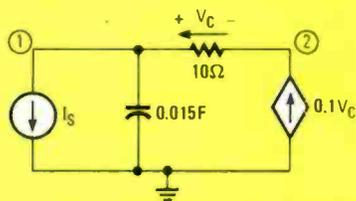
Fig. 4—Even circuits with voltage-controlled current sources such as opamps, can be analyzed by ACNAP. The polarity of the control voltage is important for proper analysis by the program, so be careful.
