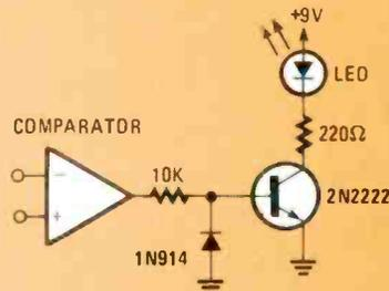
output is +8.5 volts, the transistor turns on lighting the LED. When the comparator output is -8.5 volts, the transistor is cut-off, therefore, the LED does not light.
