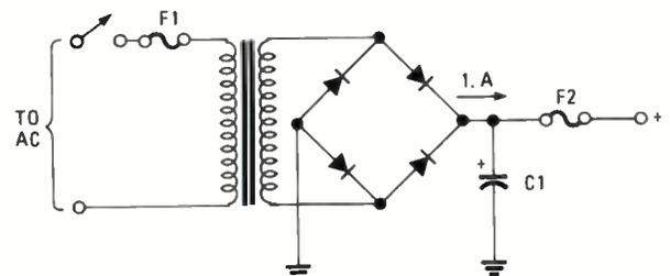
Fig. 3—A medium-acting fuse is used as F2 to provide faster action, while a slow-blow fuse is used as F1 because of the surge current provided to C1 at turn on.
