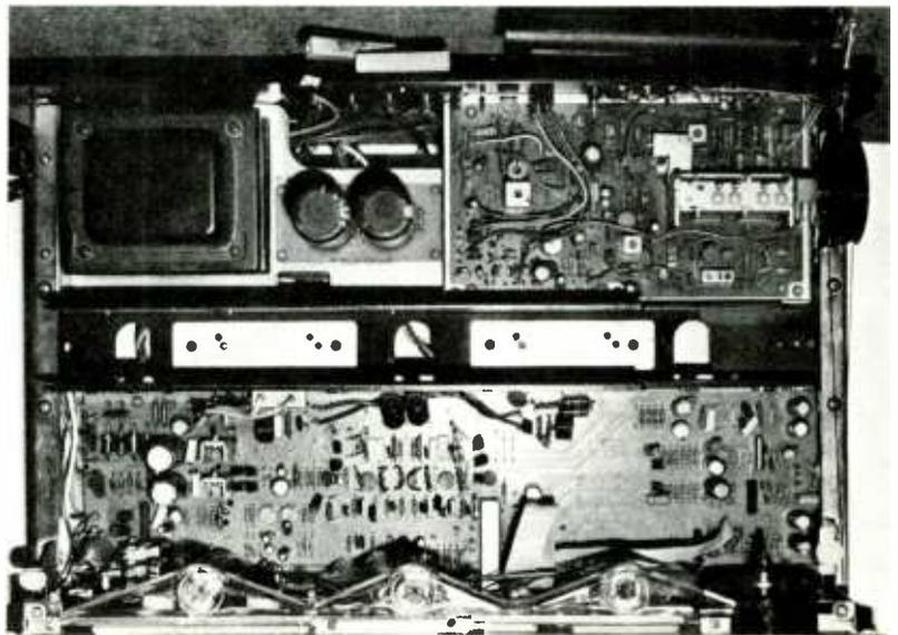
**Locate the amplifier's defective channel before testing. In many large amplifiers, the transistors and IC's are layed out in-line when the amplifier is viewed from the front.**
