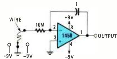
**Fig. 11—This integrator takes the flat curve defined by the constant input voltage and outputs a voltage that increases as that area under the input curve increases.**
