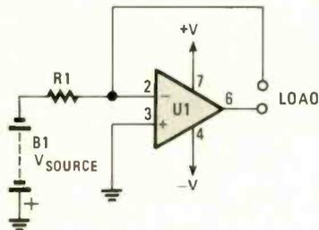
The input voltage is a stable DC reference voltage source (shown as a battery in the diagram). As with the conversion circuits discussed above, the load current ( $I_L$ ) is determined solely by the input voltage ( $V_{in}$ ) and resistor R1 ( $R_L$  has no affect) and is given by:
