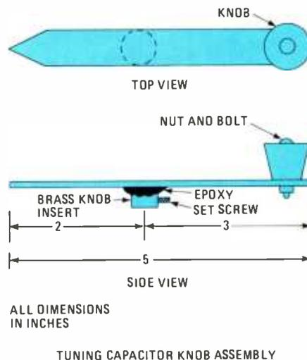
**Fig. 4—The metal pointer was constructed from a discarded brass-plated lid support; use a piece of solid brass or copper. Drill a 1/8-inch hole to secure the small radio knob and epoxy the 1/4-inch shaft insert to the under side of the dial pointer to attach to the shaft to the tuning capacitor.**
