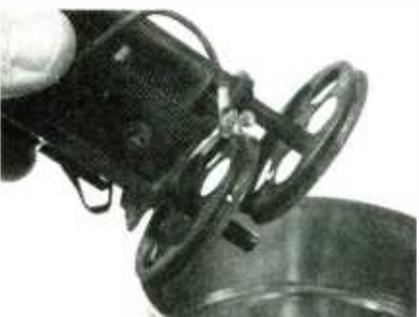
The grimy, main-tuning capacitor was bathed in mineral spirits to loosen up the encrusted dirt and dust, followed by a compressed-air blow-dry.
