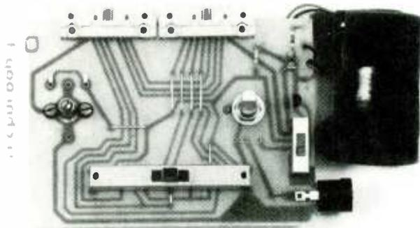
In this top view of the assembled PCB, notice that the battery is wrapped in foam rubber. That is to insulate it from other components, thus preventing shorts.
