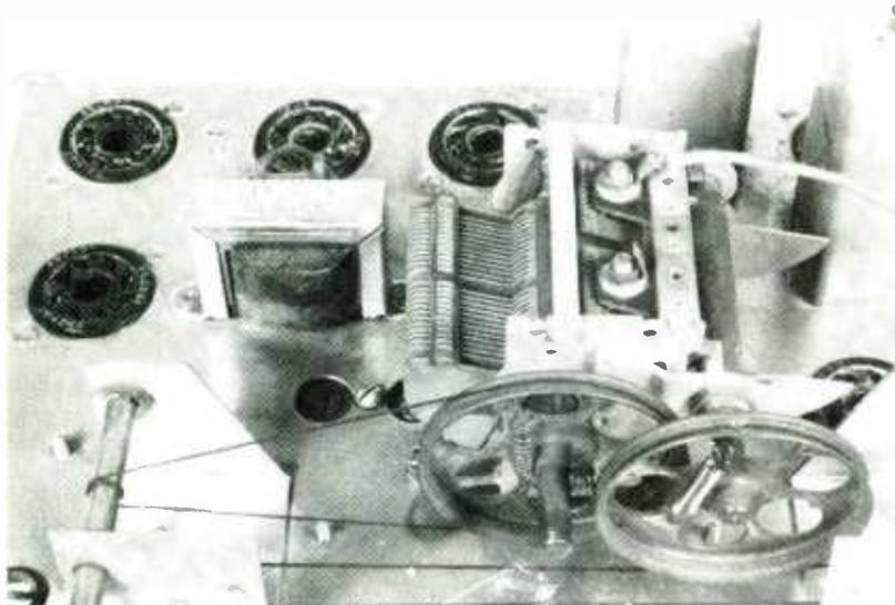
After a thorough cleaning, the tuning capacitor was placed back in place on the chassis. Note that one of the two dial cord systems has been restrung.
