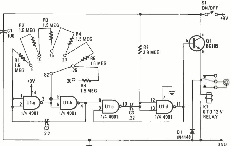
Fig. 7—The auto-advance circuit (using a 4001 CMOS quad, two-input NOR gate configured as inverters) advances the slides at intervals of 5, 10, 15, 20, 25 or 30 seconds, depending on the setting of switch S2.
