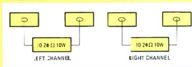
**Fig. 1—Always load the speaker terminals with 10- or 20-ohm, 10-watt resistors while servicing high-powered amplifiers. When a high DC voltage is found at the speaker terminal, turn the volume all the way down and do not connect resistor or speaker to the defective channel. Doing so might cause further damage to the amplifier, or destroy the speaker.**
