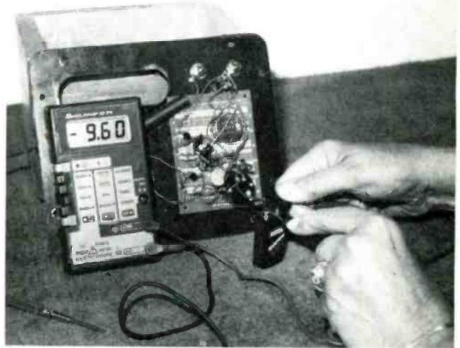
The radio pulls 10 mA with the volume turned down. If the current measurement is over 17–20 mA, suspect incorrect wiring or a leaky transistor or IC. Critical voltage and current measurements should help locate the defective component.
