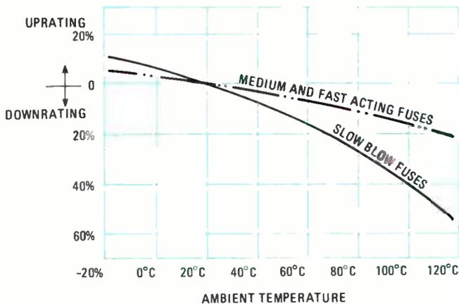
Fig. 1—A most important yet overlooked characteristic of fuse operation is the ambient temperature. As you can see, as the temperature increases the rating of a fuse drops.
