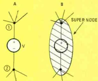
Fig. 5—A constant voltage source provides ACNAP with a way of computing the value of one node voltage by knowing another. That simplifies the matrix and speeds up analysis.
