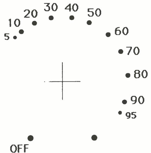
Fig. 5—To make the project easy to use, the controls should be labeled, as the author's, with a calibrated scale (like this one). Note this scale may be lifted from the page and used to adorn the project housing or you can concoct your own.
