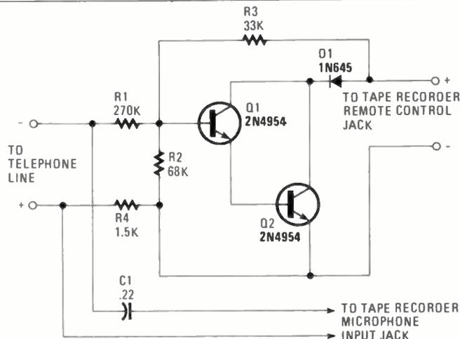
**Fig. 4—The tape recorder's switch terminals are connected to a Darlington pair (consisting of Q1 and Q2), which are used to turn the recorder on and off. The telephone's off-hook voltage (about 50-volts DC) is divided over R1, R2, and R4 so that Q1's base is negative enough to keep the recorder off. Lifting the receiver, causes the voltage to drop to 5 volts, biasing the Darlington on, which in turn, activates the recorder.**
