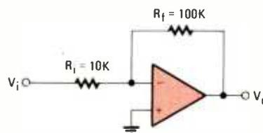
Fig. 4—The inverting amplifier requires a feedback resistor at the inverting input to channel some of the output back. That cancels some of the input signal, cutting down the gain. If one is not used, the output swings wildly.
