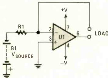
The input voltage is a stable DC reference voltage source (shown as a battery in the diagram). As with the conversion circuits discussed above, the load current ( $I_L$ ) is determined solely by the input voltage ( $V_{in}$ ) and resistor R1 ( $R_L$  has no affect) and is given by:
