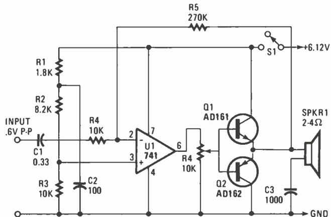
Fig. 1—The input signal is fed to the inverting input of U1 (a 741 op-amp, set up as an amplifier/buffer). U1's output is fed to the common-base leads of Q1 and Q2 (which you'll surely recognize as a push-pull amplifier). The input to the push-pull (feeding SPKR1) is controlled by R4, which serves as a volume control.
