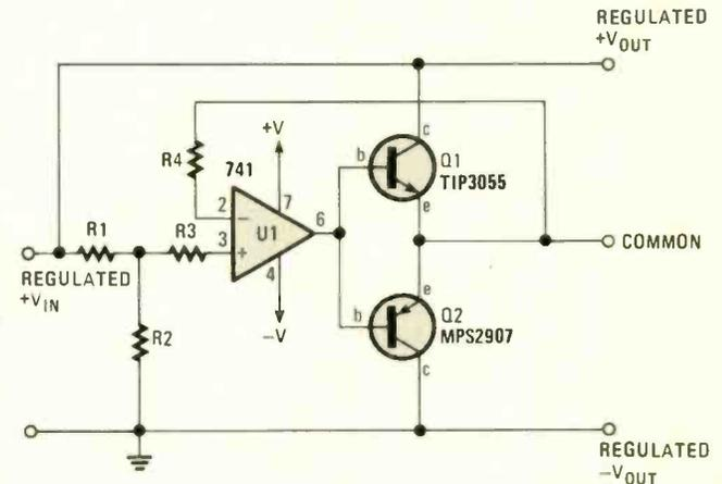
**Fig. 9—The polarity splitter allows a single-ended power supply to be used as a dual-polarity power supply, with an artificial (floating) output ground. The artificial ground should never be shorted to true ground to prevent serious shock hazard and certainly damage to semiconductors.**
