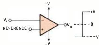
**Fig. 9—A comparator is nothing more than an op-amp with its gain wide open. Since it has no feedback resistor the output swings between the power-supply voltages.**
