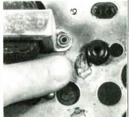
New vinyl capacitor-mounting grommets, which are much more rigid than the rubberized originals, were installed in place of the dried-out rubber ones.
