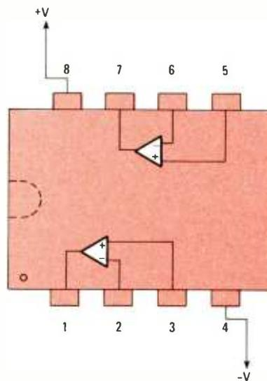
Fig. 3—This top view of the 1458 displays both op-amps in the chip. Note that both the op-amps in the package share the same power-supply pins (pin 8 and pin 4).
