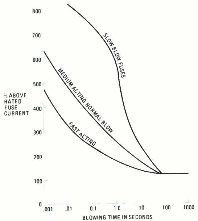
Fig. 2—Sometimes circuits are designed to run "hotter" than they are supposed to for certain applications. For that reason slow-acting fuses are needed since they tolerate overdrawn current for a length of time.
