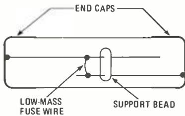
Fig. 4—This is one method of construction used to build a fuse with very-fast blowing characteristics in a 3AG case.
