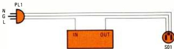
Fig. 4—This block diagram illustrates the finished *basic* circuit (with the box representing the circuit board). If your circuit is to include the neon-lamp indicator and switch S2, connect those components to the circuit, guided by Fig. 2.
