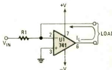
**Fig. 6—The voltage-to-current converter—also known as a transmittance amplifier—is typically used to drive relays or analog meters. The load current ( $I_L$ ) is entirely independent of the load resistance.**
