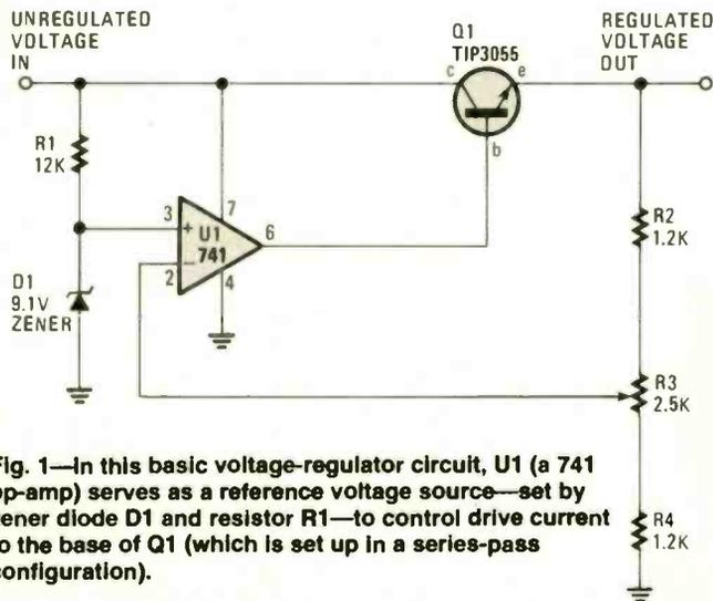
Fig. 1—In this basic voltage-regulator circuit, U1 (a 741 op-amp) serves as a reference voltage source—set by zener diode D1 and resistor R1—to control drive current to the base of Q1 (which is set up in a series-pass configuration).
