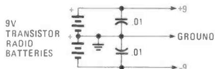
Fig. 1—This simple power-supply circuit is all you'll need to perform all the experiments in this column. Note the use of capacitors to squelch any power surges due to changing load conditions—yes, they're necessary for DC applications.
