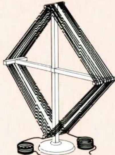
Fig. 1—The conventional loop antenna was large and unsightly. With the advent of the transistor age, miniaturization became all the rage, so the solid core antenna was born putting the air core on the shelf.
