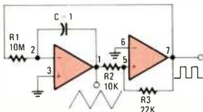
Fig. 15—Cycling the comparator output back into the integrator causes the integrator to alternately charge and discharge. Further, that causes the comparator to swing up and down, and the cycle continues creating a series of triangle and square waves to be output.
