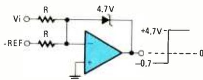
**Fig. 10—Using a zener diode as a feedback component causes the output to restrict its excursion, thus outputting clearly defined pulses. That is useful in digital circuits.**
