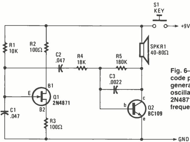
Fig. 6—The audio output of the code practice oscillator is generated by a relaxation oscillator, consisting of a 2N4871 UJT, Q1, operating at a frequency of 1.5 kHz.
