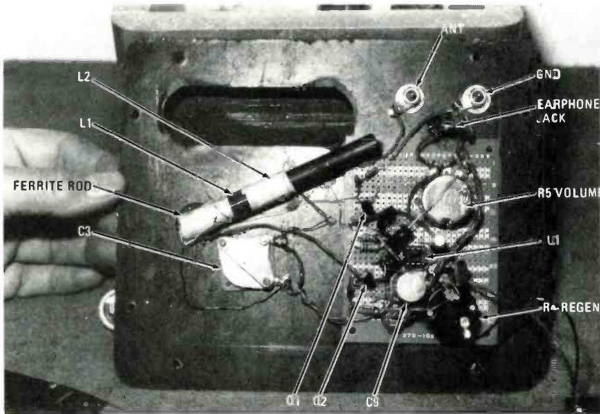
Although an IC-LS1 perfboard was used to mount all small parts, a regular perfboard may be used. The small parts are mounted into position as they are wired into the circuit.
