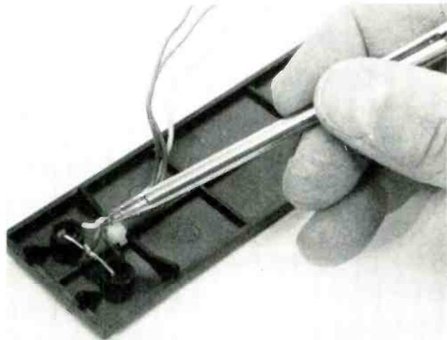
If your hard disk drive came without a front panel, you can make your own by simply installing two LED's on one of the plastic filler panels; or cut a front panel from a piece of plastic. Use a small wire tie—indicated by the pointer—to keep the wires together.
