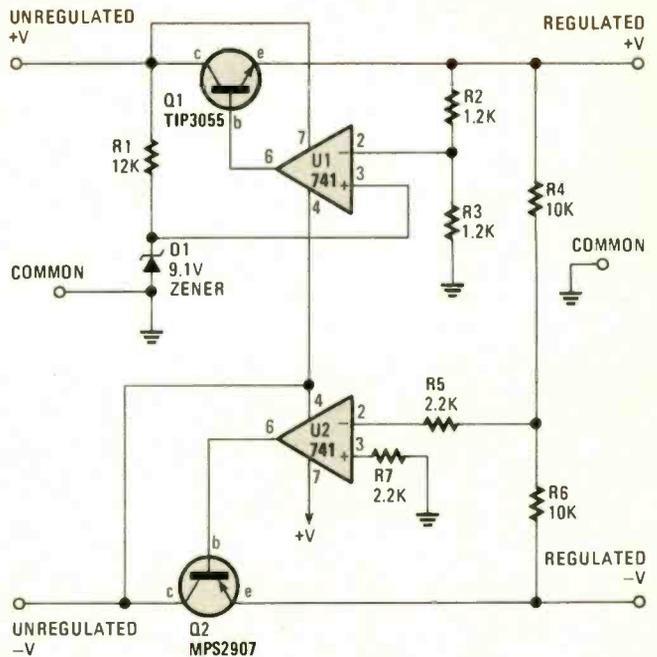
Fig. 2—This circuit is an expansion of the basic regulator circuit, amounting to a dual-polarity, op-amp based, voltage-regulator circuit that's referenced to common ground.
