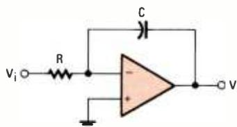
**Fig. 8—Operational amplifiers get their name from their ability to perform mathematical operations such as this integrator does. If you give it an input signal it will tell you the area of the curve defined by the input signal.**
