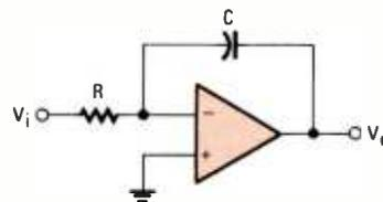
**Fig. 8—Operational amplifiers get their name from their ability to perform mathematical operations such as this integrator does. If you give it an input signal it will tell you the area of the curve defined by the input signal.**
