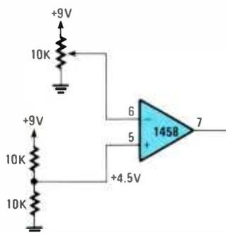
**Fig. 13—In this comparator circuit, the non-inverting input is used to receive the reference voltage, and the inverting input as the signal being tested.**
