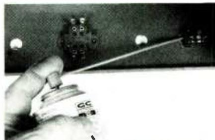
The switches and controls were treated with contact-cleaner spray, and operated several times to prevent locking prior to reassembling the chassis and panel.
