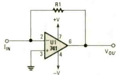
**Fig. 5—The current-to-voltage converter is simply an inverting amplifier, minus the input resistor. Output voltage is determined by the input current and feedback resistor.**
