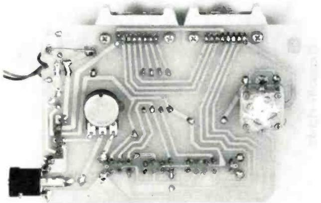
As you can see the tuning capacitor and potentiometer are mounted on the foil side of the board. Note also how the contact strips on the coaxial connector hold it in place.
