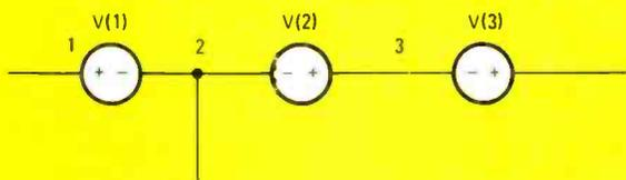
**Fig. 2—Voltage sources must be assigned node numbers in consecutive order for proper processing by the program. Notice that their polarities have no effect on numbering.**
