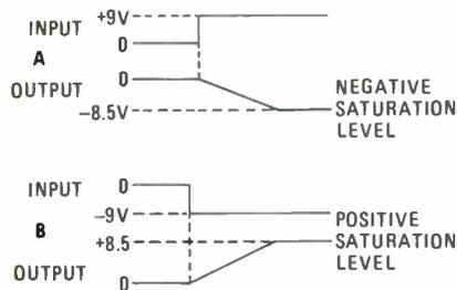
**Fig. 12—Of course the output of an integrator can't reach infinity no matter how long the input signal is left on. The output is limited by the negative (A) and positive (B) power-supply values. A perpetual motion machine it's not.**
