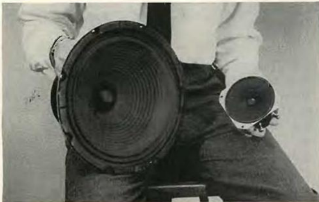
These two speakers illustrate the differences in cone structure and area discussed in the text. The speakers are a twelve-inch woofer (Cletron Cathedral Series, 30-5000 cycles) and a four-inch tweeter (also Cletron Cathedral Series, 1800-18,500 cycles).
