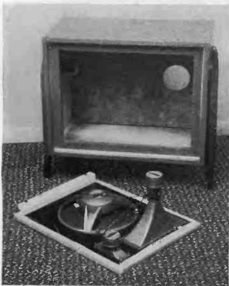
Bass, mid-range and treble speakers are mounted on the front panel, which is the removable part of the Lancaster enclosure (left). The two crossovers used in the three-way system are fastened securely to one side of the rigid cabinet by their level controls (center). The front panel is unscrewed and re-fastened by reaching through a temporarily unsealed opening in the flexible rear panel (right).
