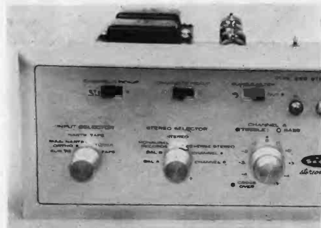
These two views of the panel of the Scott 299 show the major control functions. Concentric shaft individual channel tone controls appear on either side of the brand name decal. Two separate magnetic inputs are accommodated by separate slide switches.
