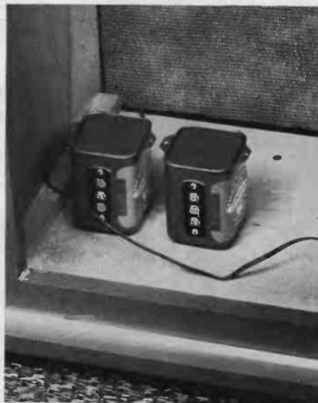
Bass, mid-range and treble speakers are mounted on the front panel, which is the removable part of the Lancaster enclosure (left). The two crossovers used in the three-way system are fastened securely to one side of the rigid cabinet by their level controls (center). The front panel is unscrewed and re-fastened by reaching through a temporarily unsealed opening in the flexible rear panel (right).
