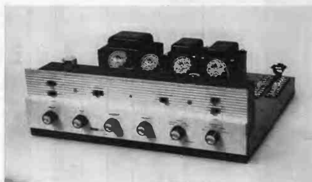
Harman-Kardon A-250 doubles up on equalization switch to provide for tape compensation at 3¾ and 7½ ips speeds. It is one of the few amplifiers purposely designed to permit use of two different pairs of stereo loudspeakers. Input jacks are located on top of chassis deck. Plastic cable clamp at lower left corner is a thoughtful addition on the part of manufacturer.
