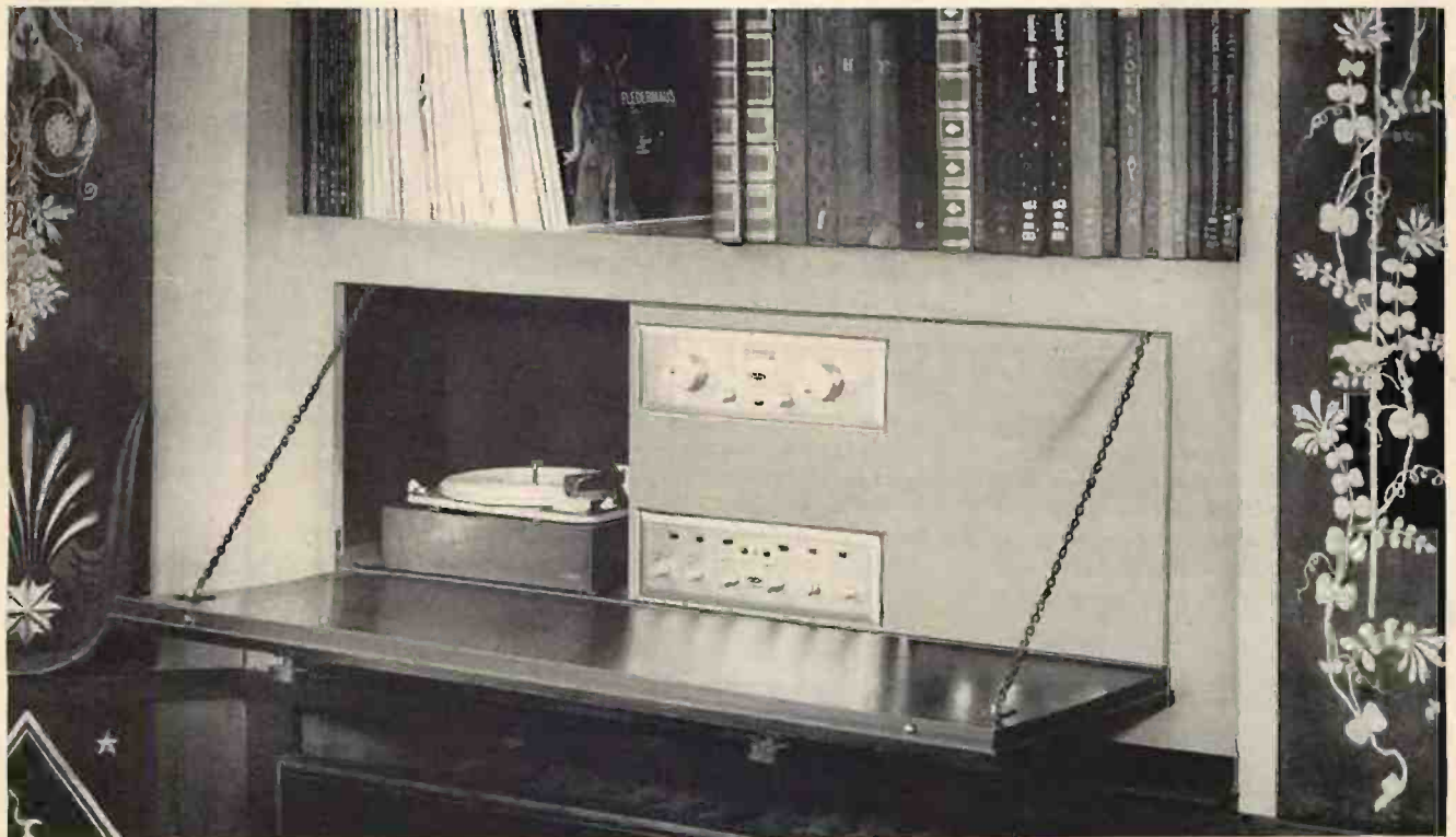
The main installation of the Schulers' music system. Equipment includes a Scott 299B stereo amplifier, a Scott 330C stereo tuner, and a Dual 1006 record changer with an Audio Empire 108 cartridge. The space behind the panel at the right is occupied by an EICO HF-22 basic amplifier, which supplies power to the extension speakers.
