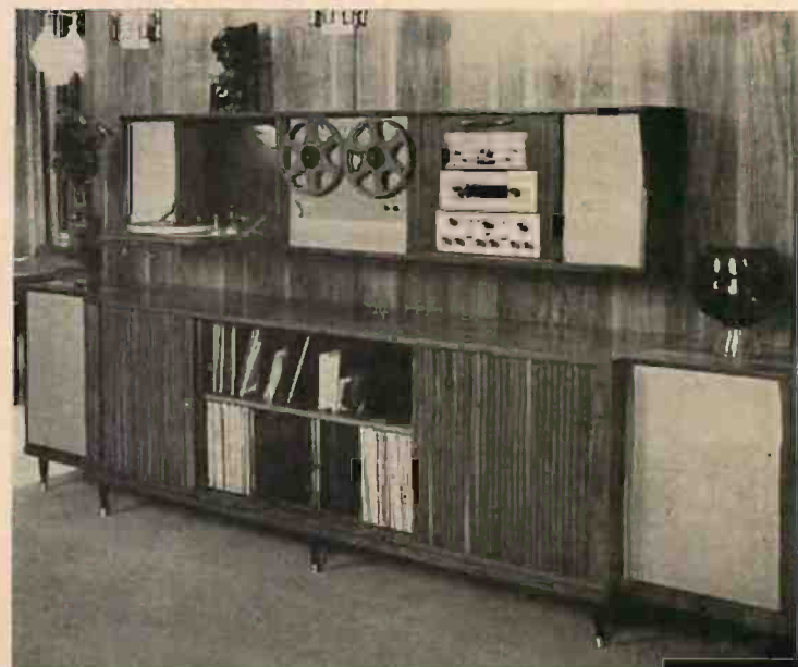
To gain floor space for large speakers and record storage, Hardoff designed wall-suspended equipment cabinet.
