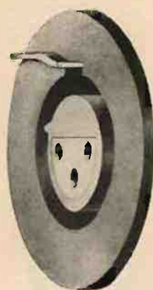
Recorders that have a three-circuit microphone input of the type shown here usually have enough gain to be used with professional-type low-output microphones.
