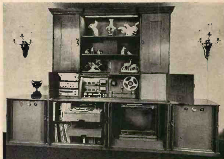
The owner of this installation insisted on preserving period furniture appearance, so tambour doors that can be closed over the entire system were provided.
