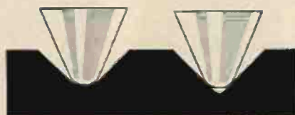
ROUNDED BOTTOM OF OLD MICRO-GROOVE DOES NOT GRIP SMALL STYLUS
