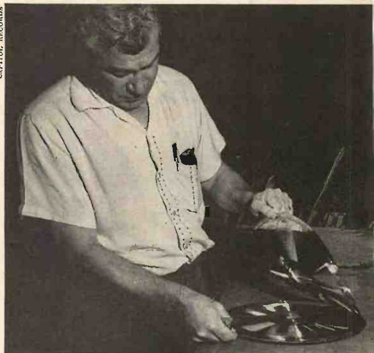
Separating the master from the lacquer is a crucial operation.
