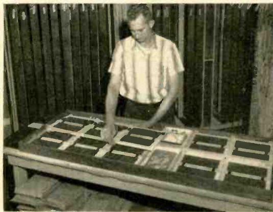
KLH's Model 9 consists of two matched full-range electrostatic speakers. Each of the handmade units has twenty sound radiators.
