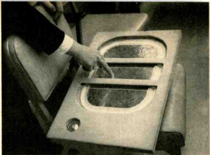
Polystyrene-foam cones are employed in the ADC woofer pictured above (also note the aluminum-foil front surface, used for improved coupling to the air) and in the IMF woofer, below.
