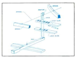
A simplified view of the harpsichord's basic mechanism for plucking a single string. See diagram below for a more detailed view.
