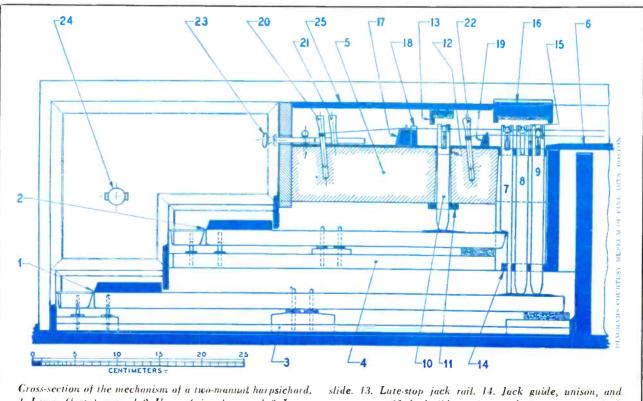
Cross-section of the mechanism of a two-manual harpsichord.
