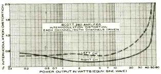
is another demonstration that transistor amplifiers do not have to show a rise in distortion at low power levels. The averaged IM distortion of the 260 was below 0.4 per cent up to about 16 watts output, rising to 1 per cent at about 40 watts and 2 per cent at about 55 watts per channel (equivalent sine-wave power).
