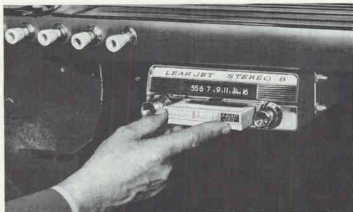
Two versions of the tape players that take the Lear Jet "Stereo 8" cartridge are shown above. The machine above right is offered by Ford as a built-in optional accessory. The machine above left is a "hang-on" type designed for installation in any car. The player at right is by Martel and is intended to fit over the car's transmission hump. The built-in speakers can be raised or lowered and the unit is powered by plugging it into the cigarette-lighter receptacle on the dashboard.
