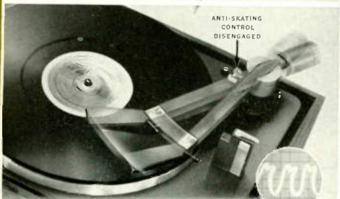
4 "Now you can actually watch the strength of the skating force. I start the Lab 80, but flip the anti-skating control over and out of operation. Note that as soon as I put the stylus on the grooveless record, the arm moves rapidly... with force, toward the center."
