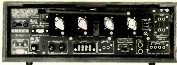
Unusual features of the 387's rear panel include phono-jack outputs for the main stereo speakers and a connector for the detachable a.c. line cord. The power transistors are normally covered.
