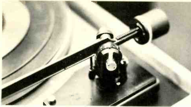
The Dual 1215's stylus-force adjustment (a knurled, calibrated ring on the pivot assembly) simultaneously sets the anti-skating compensation. The counterweight rotates for tone-arm balancing.
