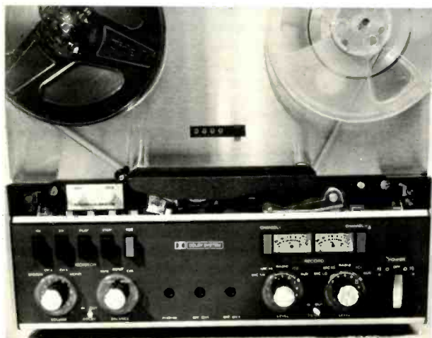
With the head cover flipped down for tape loading, the Dolby calibration controls are seen in the location occupied by the reel-motor and monitor-amplifier switches on the non-Dolby A77.
