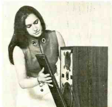
Install speakers with quick disconnect wire harness and press grille against Velcro fasteners.
