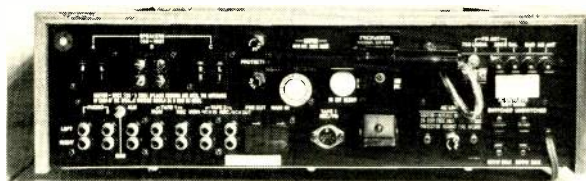
The two sets of tape-monitor jacks on the 626's rear panel will take two tape machines, or one machine and a quadrasonic decoder. Special plugs are provided for the speaker-output sockets.
