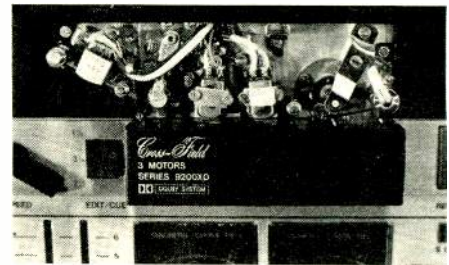
The head layout of the 9200XD. The cross-field head is underneath the lower cover.
