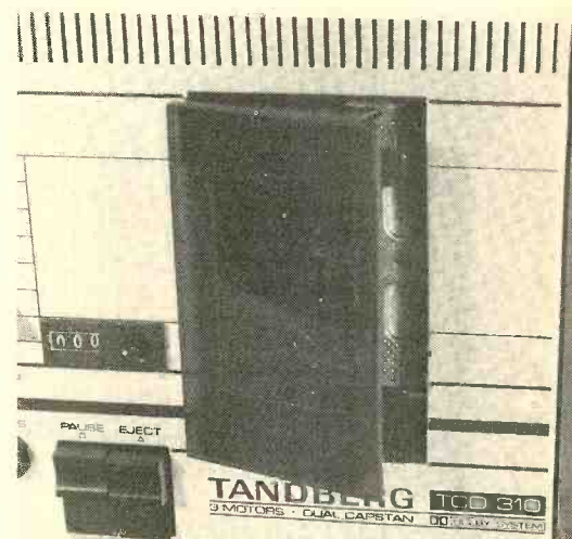
The TCD-310's tape-well cover holds a cassette in integral slots. The clear top plate of the cover snaps off to permit easy head access.
