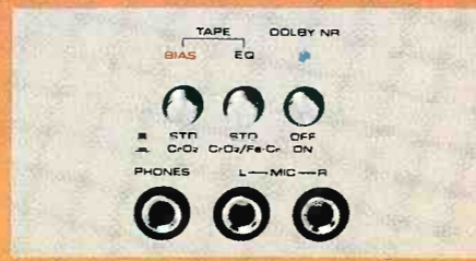
Separate bias & equalization switches for any type of cassette tape.
