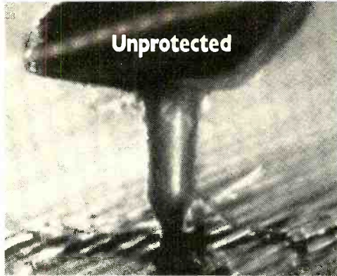
Magnification shows the record vinyl wearing away.
