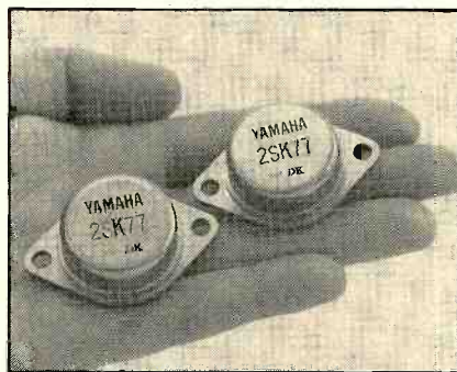
One power FET can replace as many as four or five conventional output transistors. The photo indicates their quite substantial size.
