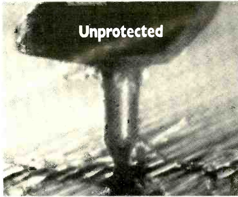
Magnification shows the record vinyl wearing away.
