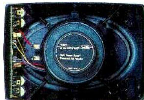
Rear view of the Power Bass, showing built-in amplifier. When added to any tape player or radio, the Subwoofer bi-amplifies the system, improving the dynamic range and reducing distortion.
