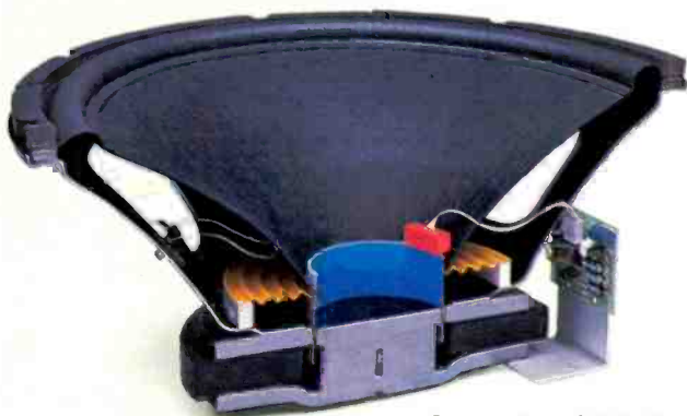
Cross-section of ULD-15 driver with accelerometer in housing (red) mounted on voice coil (blue). Circuit board contains associated HGS electronics.
