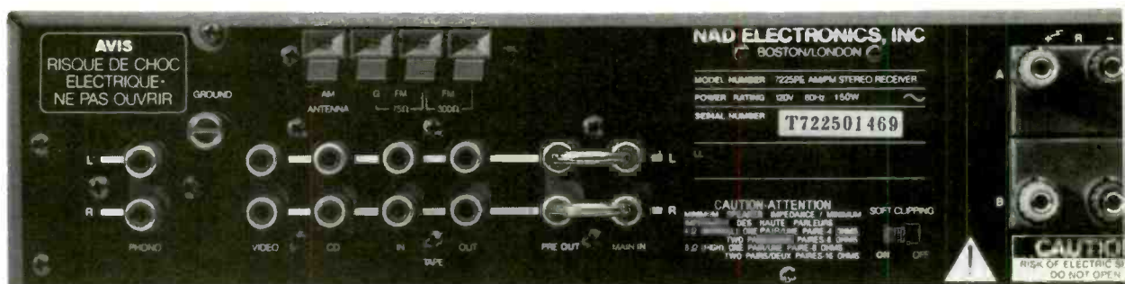
The rear panel contains additional controls and connections, including the Soft Clipping switch, speaker impedance selector, gold-plated phono-in jacks, heavy-duty binding-post speaker terminals, and preamp-out/main-in jumpers for system expansion.
