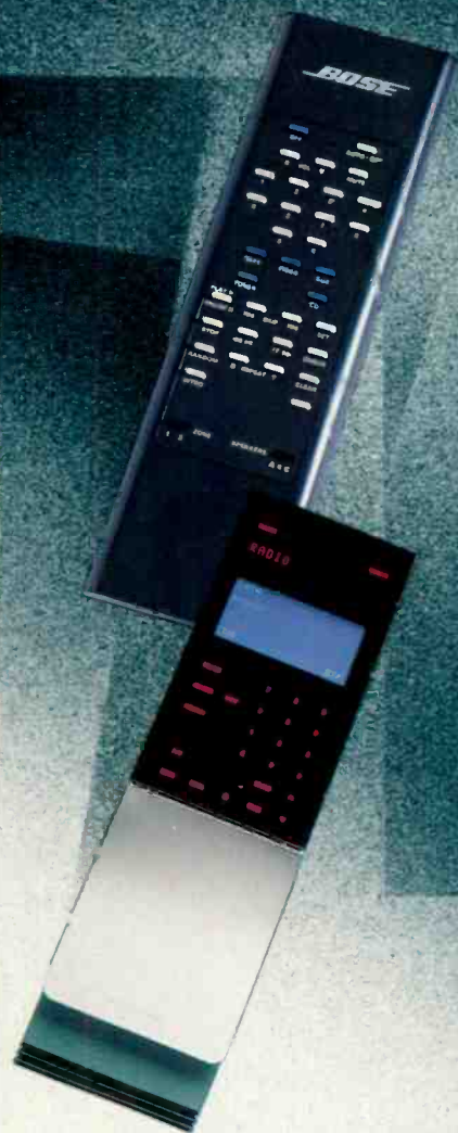
Bose uses a dedicated radio-frequency remote for its Lifestyle Music System. Bang & Olufsen's amazing $1,000 Beolink 7000 interactive remote operates B&O components and displays status information sent back from them.
