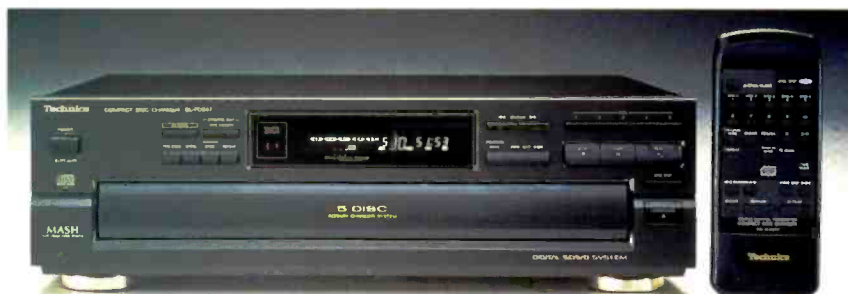
The Technics SL-PD847 five-disc carousel changer ($230) lets you swap four discs while the fifth is playing. An ID Scan mode previews each track on a disc, playing the loudest (and most easily recognized) passage of each song for 10 seconds.
